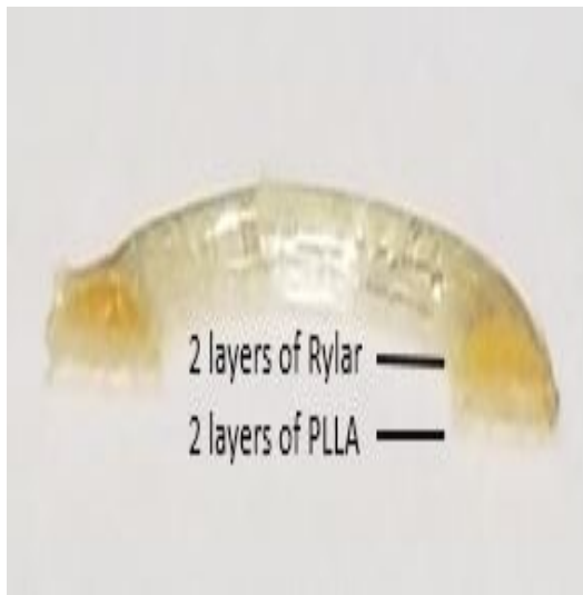
(a) Continuously printed composite scaffold cross section
