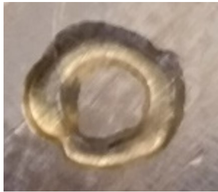
Figure 3.9: Unsuccessful printing of Rylar due to lower UV intensity
