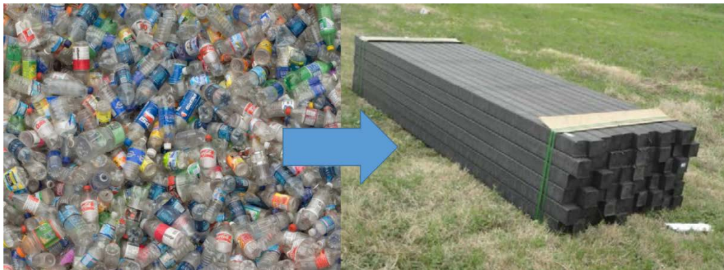
Figure 2. 60 Recycled Plastic Pins (Hossain et al., 2017).
