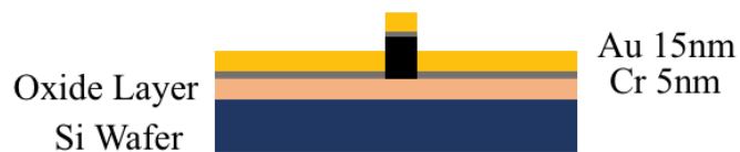
Fig 29 Schematic side view after deposition
