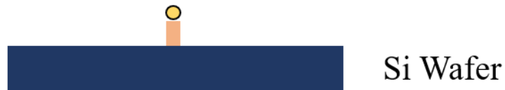
Fig 38 SiO 2 nanopillar formed via RIE
