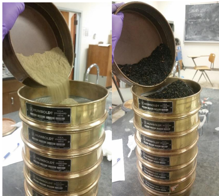
Figure 3- 28 Pouring the sample, soil (left) and rice hull ash (right) into top sieve
