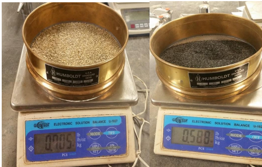
Figure 3- 30 Sieves with the retained sample
