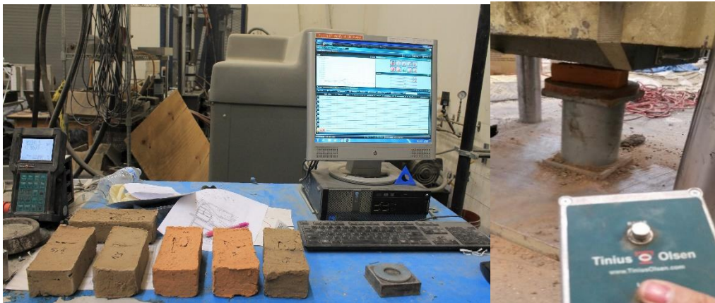
Figure 3- 45 Proterm, computer running software (left) and cross-head controller (right)
