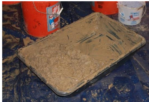
Figure 3- 35 Soil dough for making the bricks
