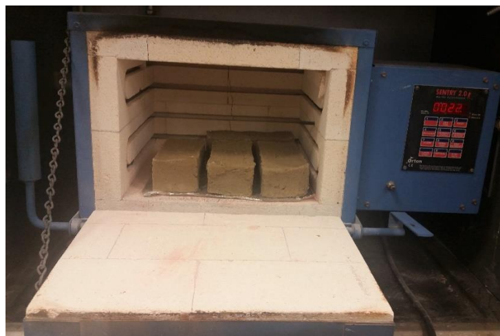
Figure 3- 41 Firing bricks in the muffle furnace
