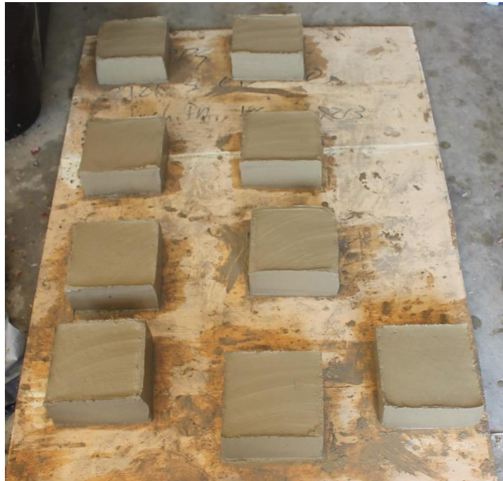
Figure 3- 53 The sample for thermal conductivity measurement.
