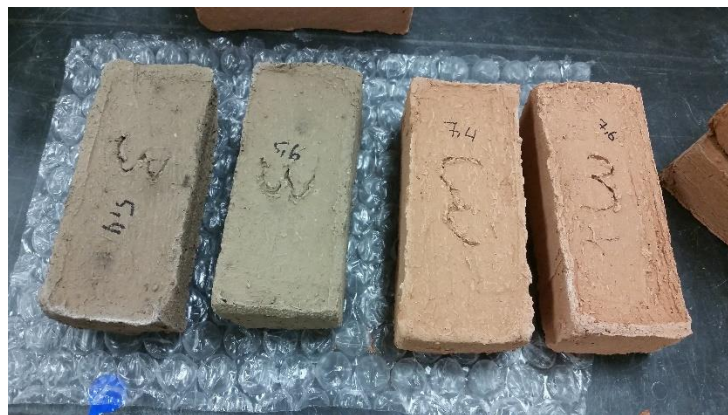
Figure 3- 42 The same proportion of brick fired at different temperatures and times
