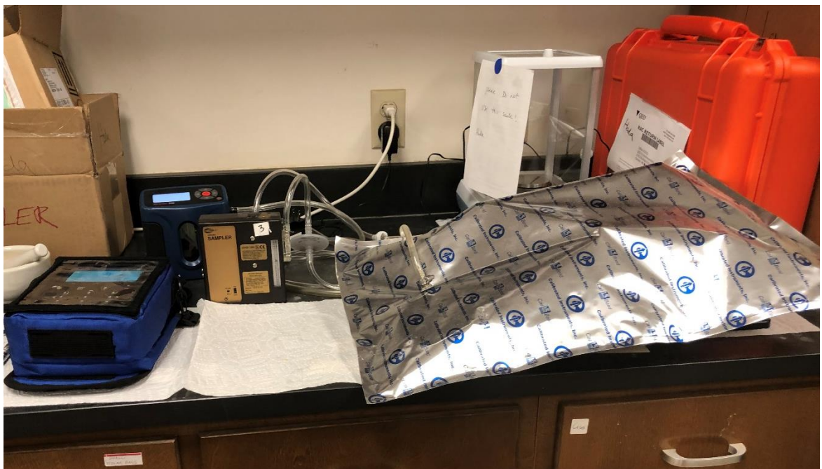
Figure 3- 91 Volume measurement instruments, Calibrator & SKC Sampler
