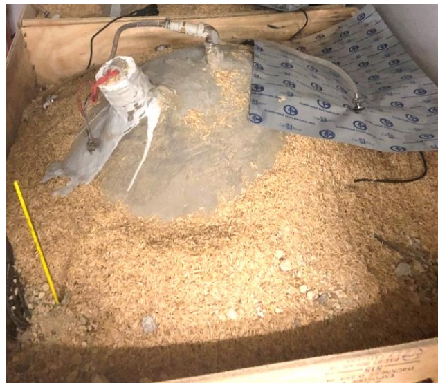
Figure 3- 79 Earth filling outside the reactor
