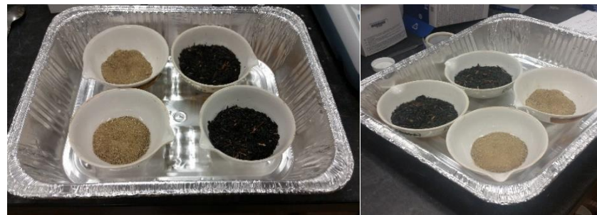
Figure 3- 12 Samples before (left) and after 24 hours drying in an oven at 108°C (right)
