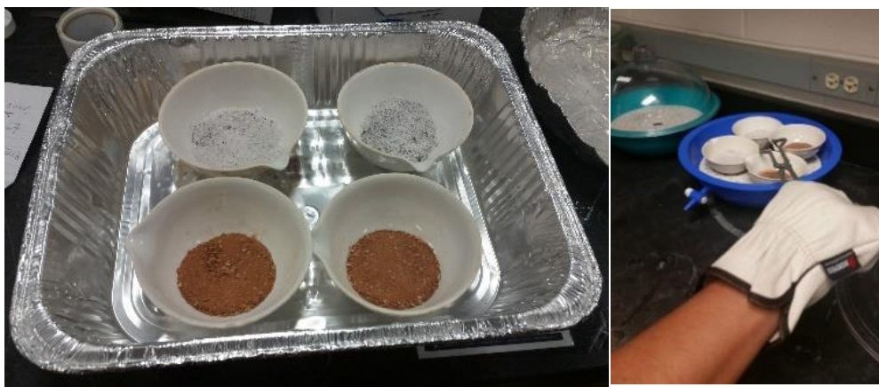
Figure 3- 14 Sample after 1 ½ hour burning in the furnace at 650° C
