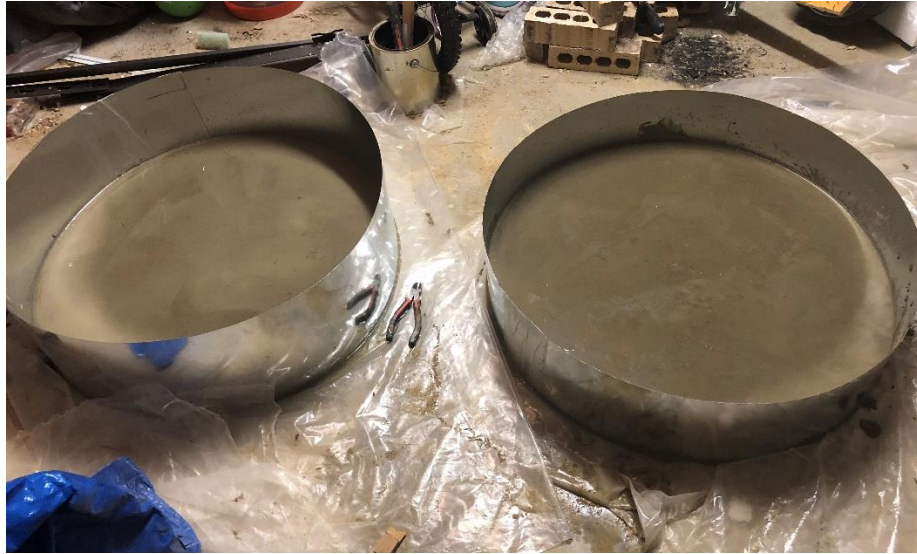
Figure 3- 58 Curing of concrete
