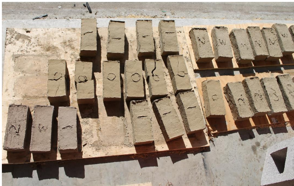
Figure 3- 39 Bricks drying in the sun
