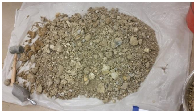
Figure 3- 8 Drying the soil to remove moisture
