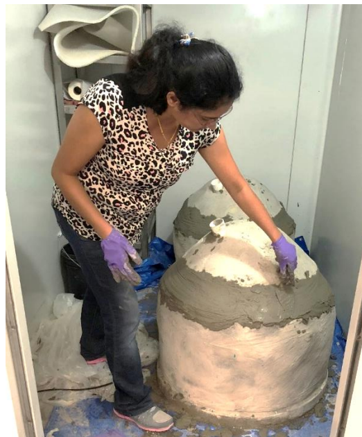
Figure 3- 73 Attached the gas holder with the circular reactor
