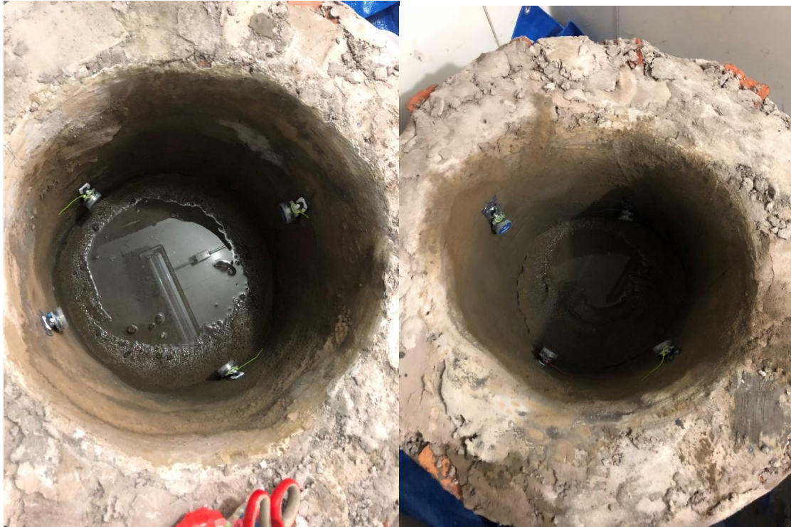
Figure 3- 71 Attachment of temperature sensors inside the reactors
