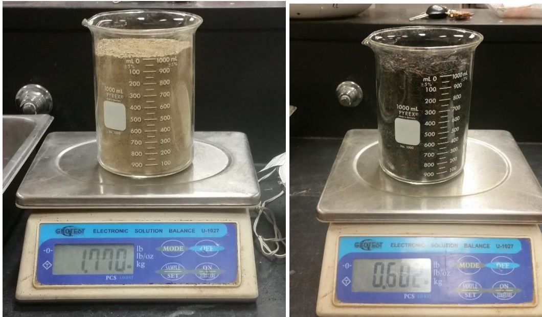
Figure 3- 25 Beaker with sample soil (left) and rice hull ash (right)
