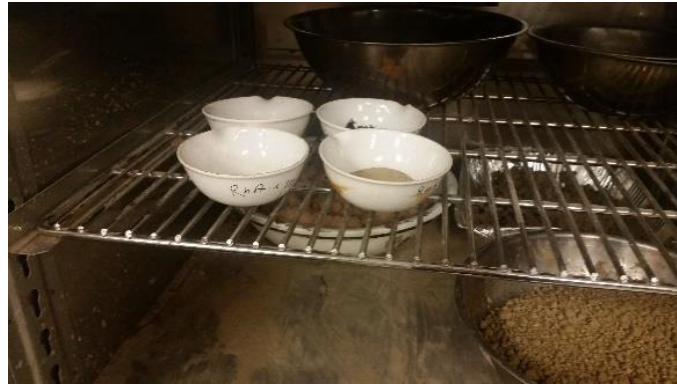
Figure 3- 11 Samples in the drying oven for moisture content test
