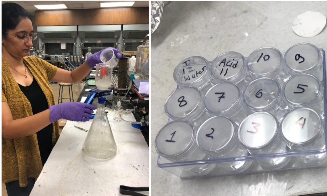
Figure 3- 22 Eluate filter and samples prepared for heavy metal analysis
