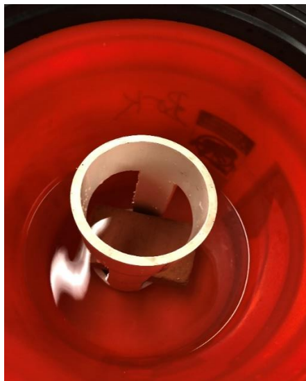
Figure 3- 19 Sample with the holder placed into the leaching vessel.
