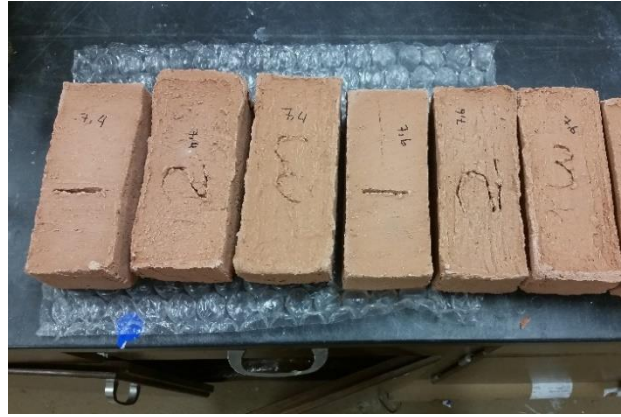
Figure 3- 43 Bricks with different mixing proportions after burning at 700 ° C for 4 and 6 hours
