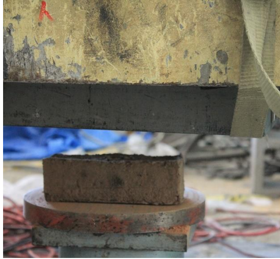
Figure 3- 46 The specimen in between plate and cross head
