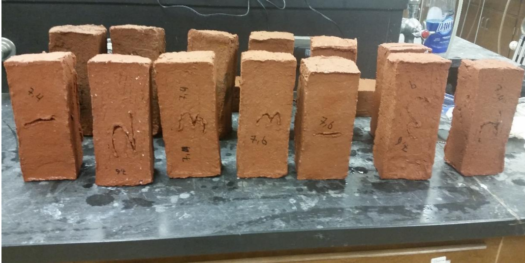
Figure 3- 51 Specimen removed from the water bath
