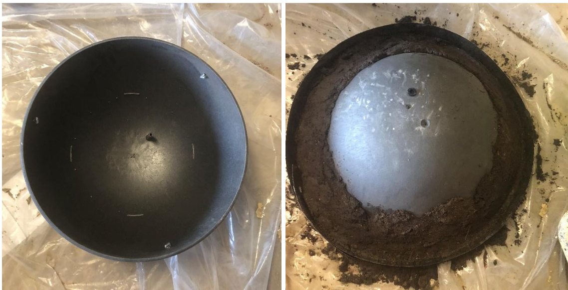
Figure 3- 60 Planter to use as a frame for casting dome-shaped gas holder
