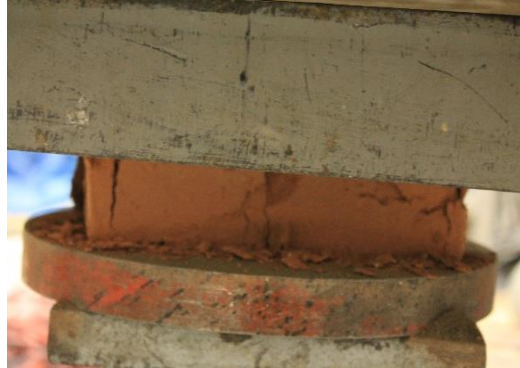
Figure 3- 48 Sample after the ultimate load was reached
