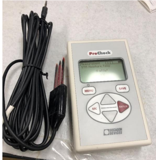
Figure 3- 80 Temperature and soil moisture sensors (Pro Check Decagon)
