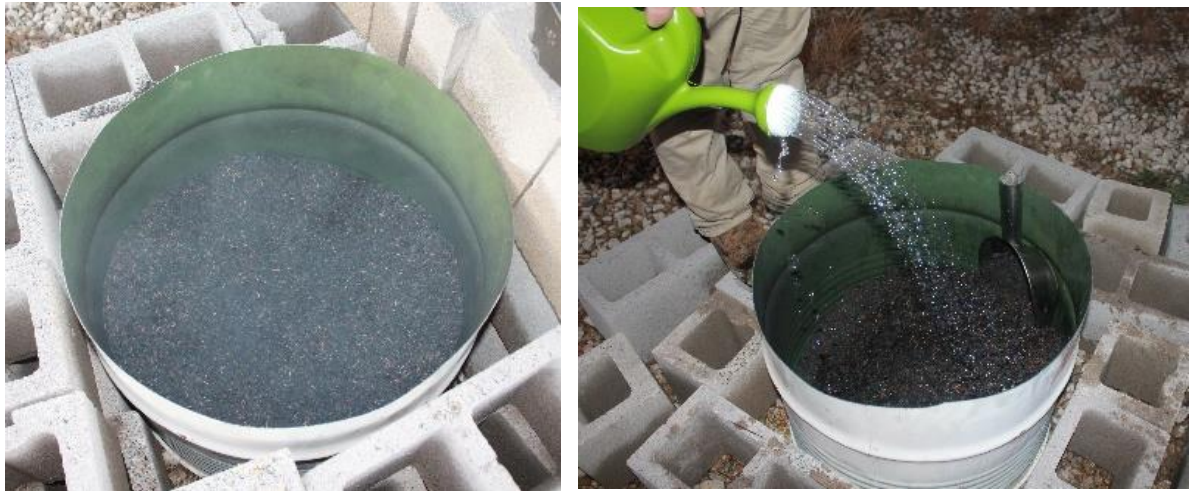
Figure 3- 6 Rice husk charcoal after burning (a), spraying water (b)
