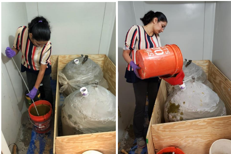
Figure 3- 84 Mixing and feeding waste to the reactor
