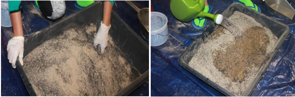
Figure 3- 34 Manually mixing soil and RHA (left); adding water to the sample (right)
