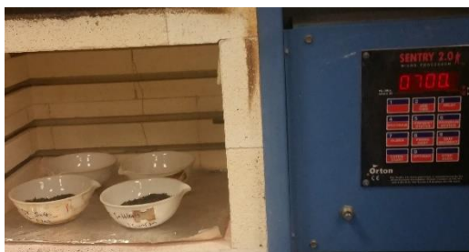
Figure 3- 13 Samples in the muffle furnace
