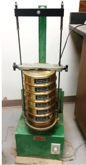
Figure 3- 29 Series of the sieve on a mechanical shaker
