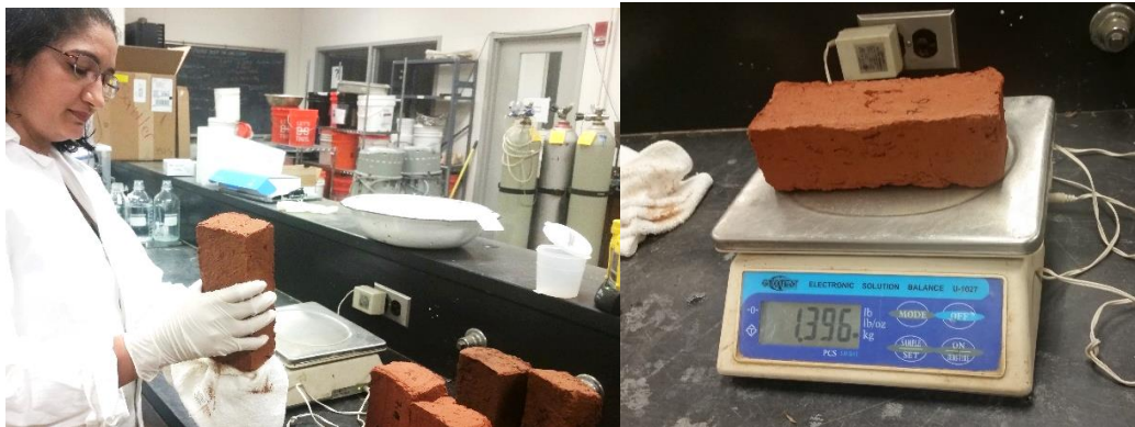
Figure 3- 52 Specimen cleaned (left) and reweighed (right)
