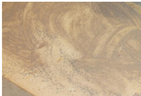
Figure 3- 36 Dry coarse-grained soil sprayed on wooden board
