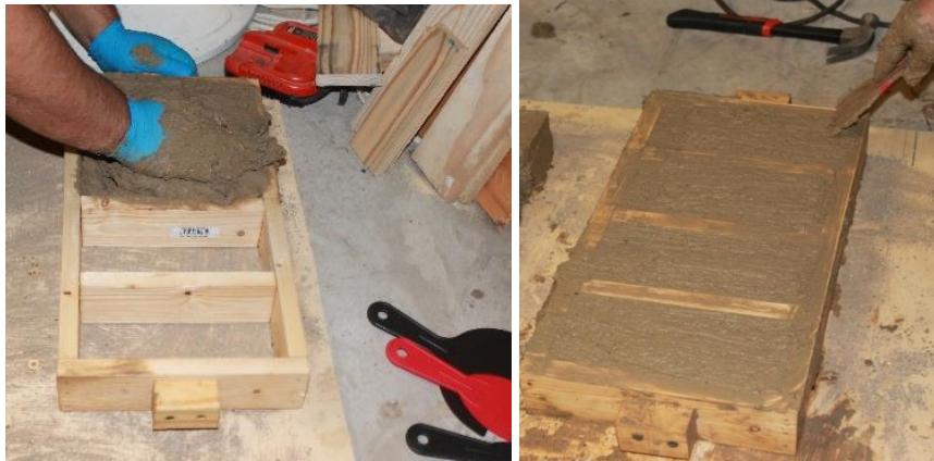
Figure 3- 37 Packing dough into a mold (left) leveling the edge (right)
