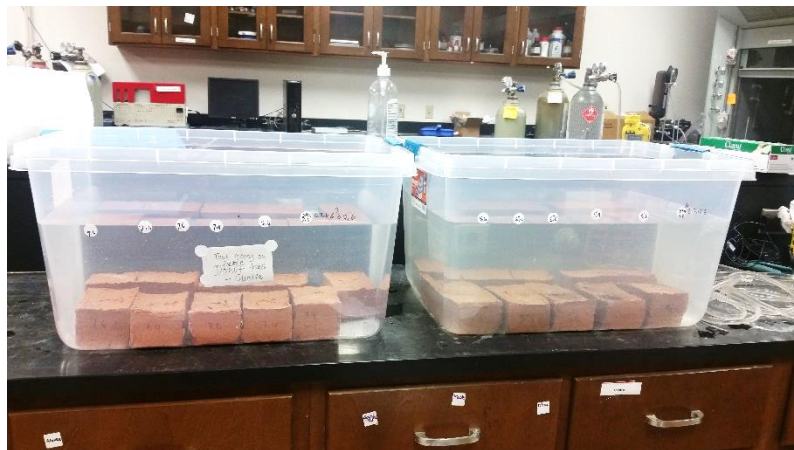
Figure 3- 50 Specimens immersed in water for 24 hours
