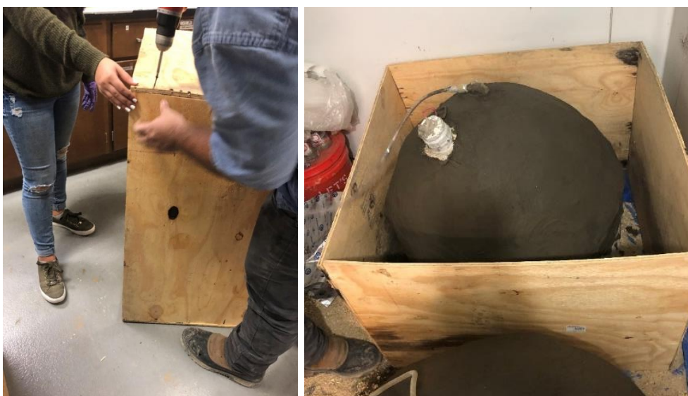
Figure 3- 78 Preparation of the plywood box to keep the reactor
