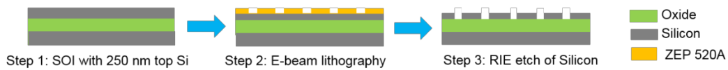
Figure 3-1: Process flow for fabrication of PCS on SOI substrate with t = 250 nm.
