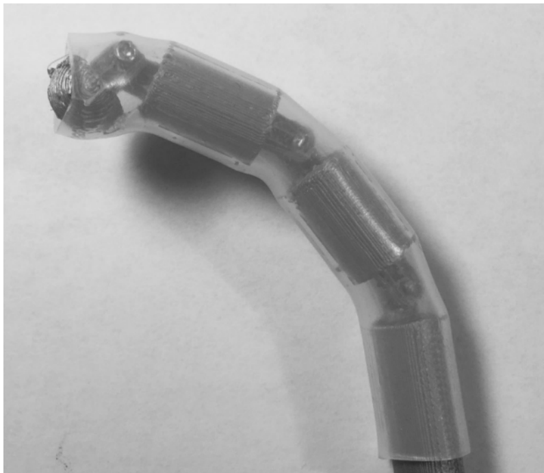
Figure 5.4: Image Showing 3D Printed and Assembled Flexible-Continuum Part with Actuation Load on One Tendon at Scale 1 : 3.47
