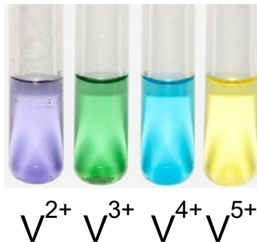
Figure 2-5 Different oxidation states of vanadium ions
