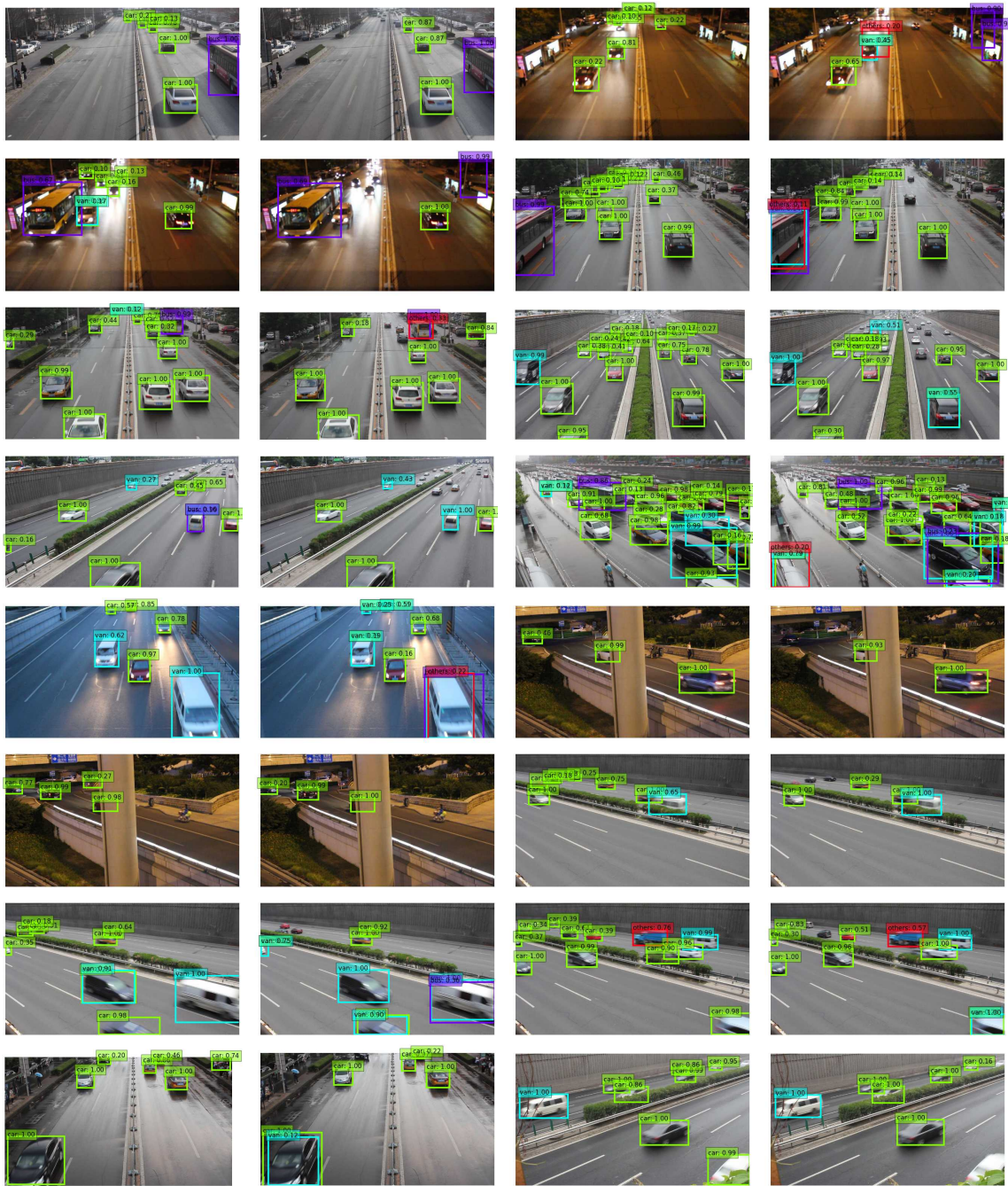
Figure 3.18: Curated examples of DiCSSD (left) and SSD (right) on DETRAC test set.
