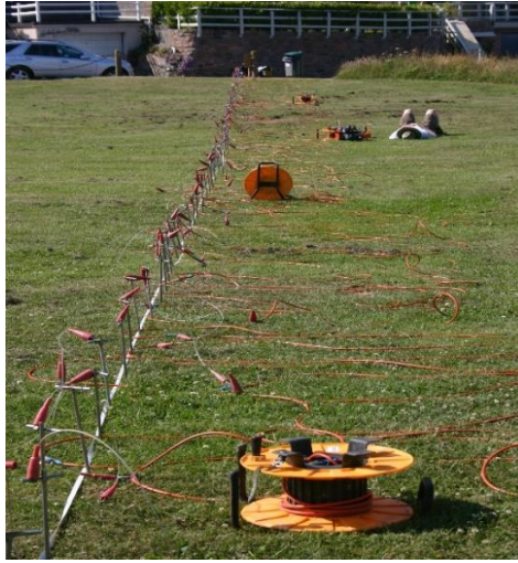
Figure 2.21 Field measurement of soil resistivity
