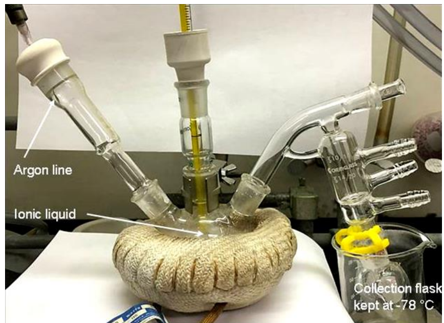
Figure 4-1 The Experimental setup for the collection of volatile fragments
