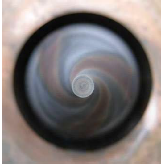
Figure 1.9. Evidence of exit swirl on aerospike nozzle [120].
