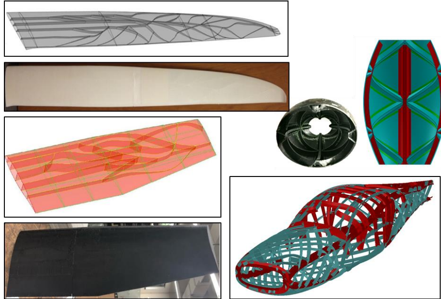
Figure 2-2 Examples of Stiffness Tailoring through Additive Manufacturing 12
