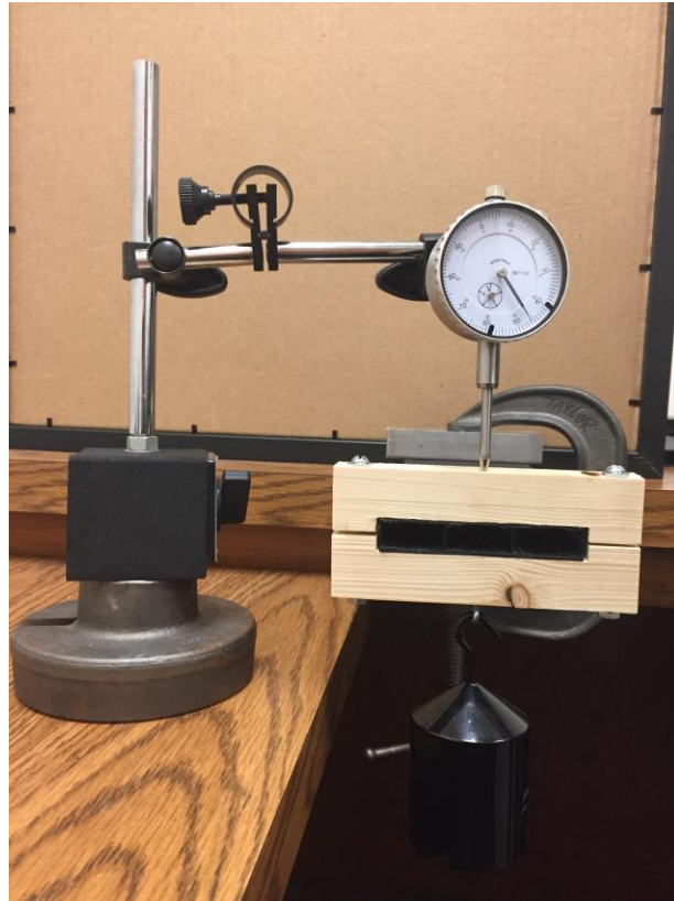
Figure 3-13 Cantilever Bend Test Setup
