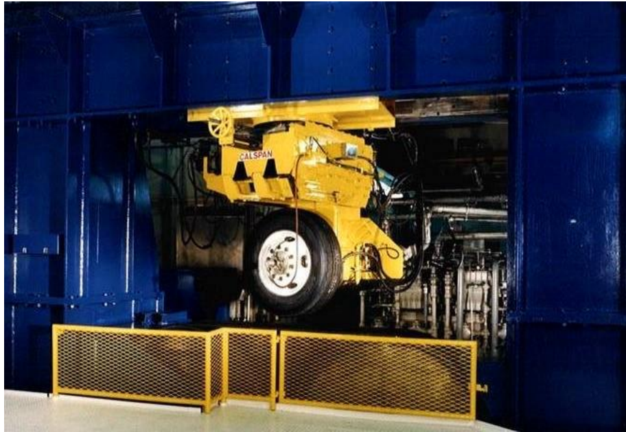
Figure 5: Main testing machine Calspan, TIRF.
