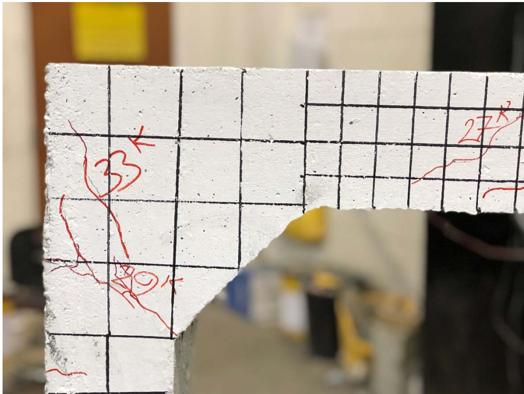
P13. Flexural cracks in connection of slab and wall- f'_c = 4.8 ksi
