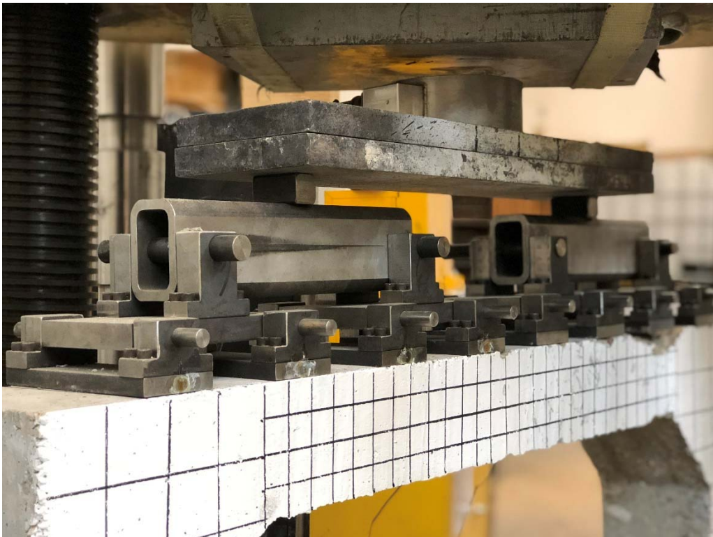
P11. Applying the framework on the top of the box culverts- f'_c = 4.8 ksi
