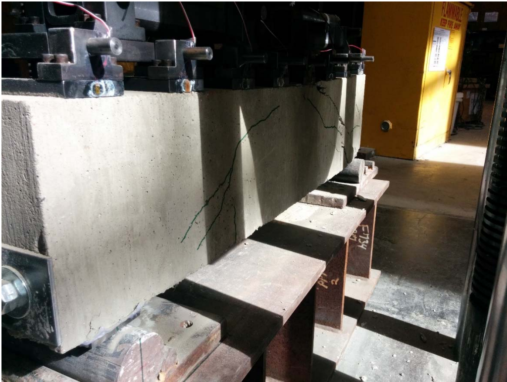
P5. Shear Cracking (continued)
