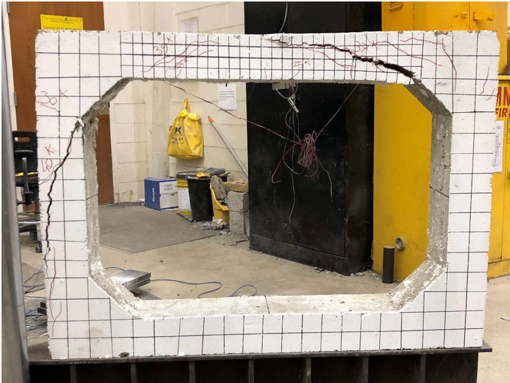
P15. Shear cracking- f'_c = 4.8 ksi (continued)
