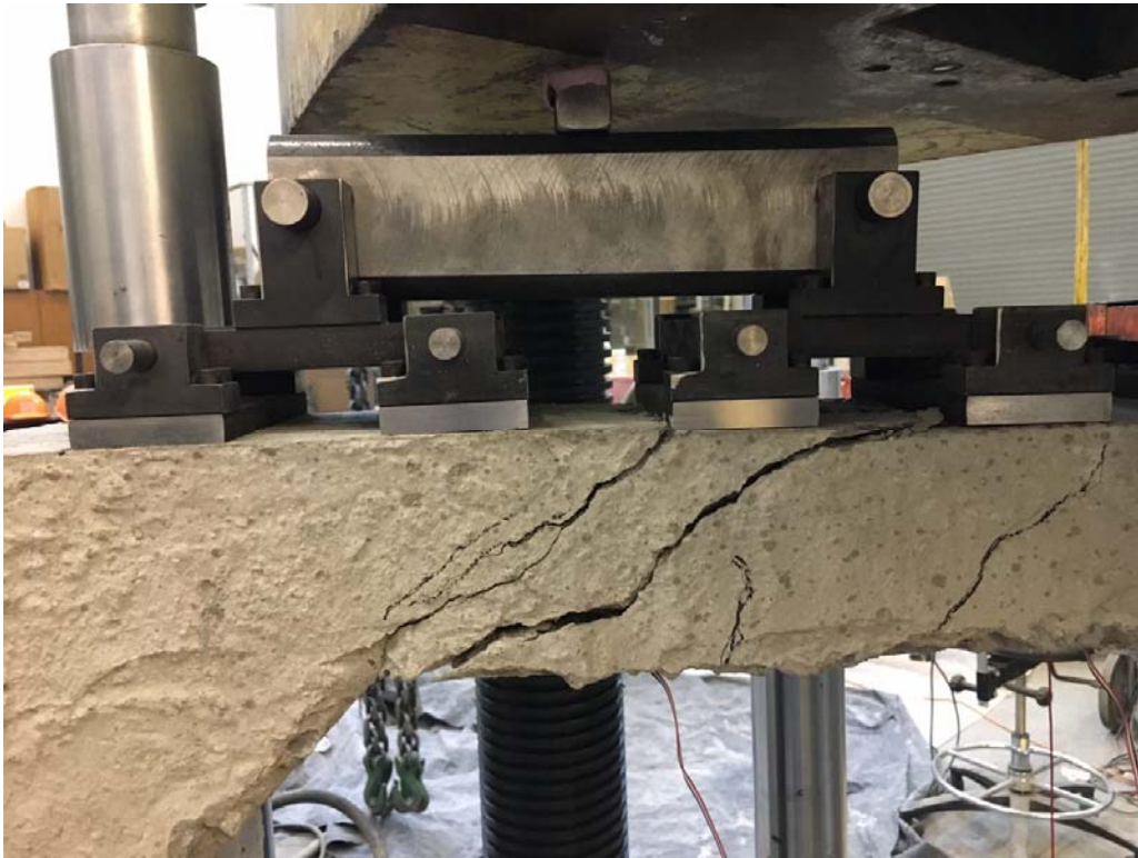
P8. Shear cracking- f'_c = 6.5 ksi (continued)
