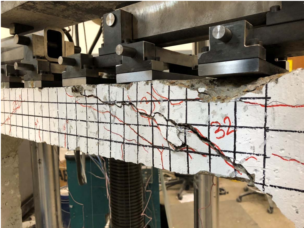
P15. Shear cracking- f'_c = 4.8 ksi
