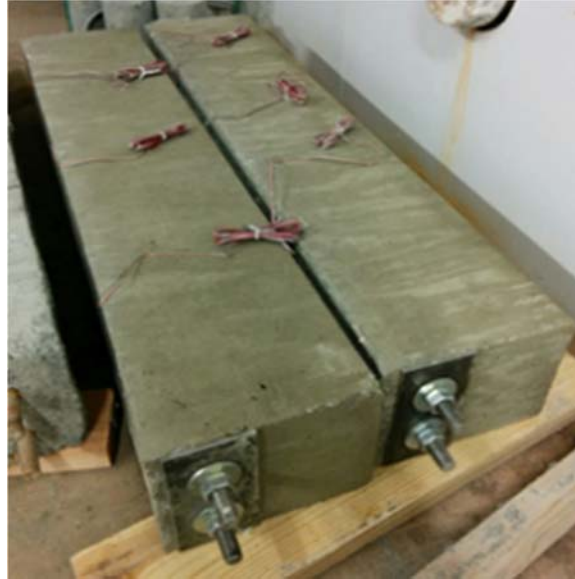
Figure 19. Beam specimens prepared for tests in moisture chamber
