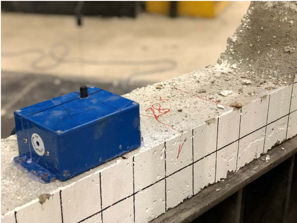
P14. Minor cracks in the bottom slab- f'_c = 4.8 ksi
