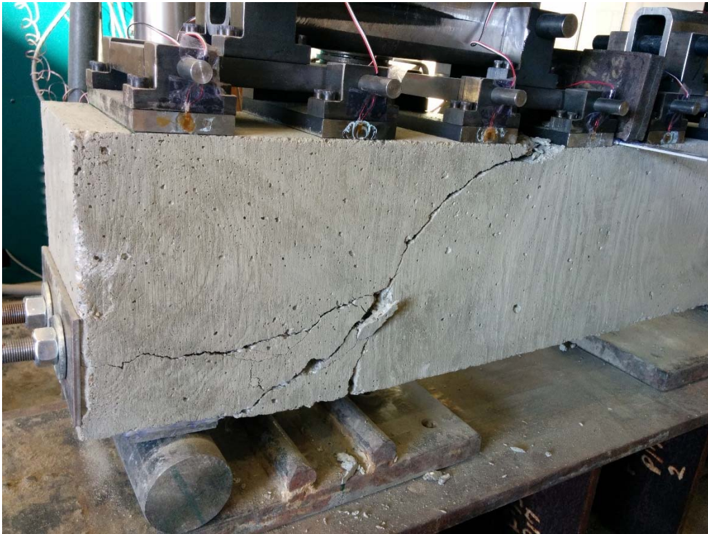
P5. Shear Cracking (continued)
