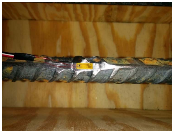
Figure 22. Strain gauge installation
