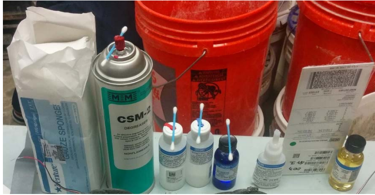
Figure 43. Chemicals for strain gauge installation
