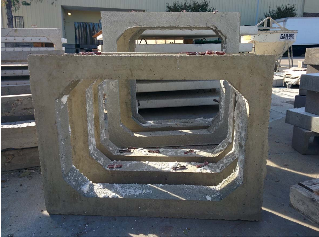
P9. Building box culverts for the second series of testing- f'_c = 4.8 ksi
