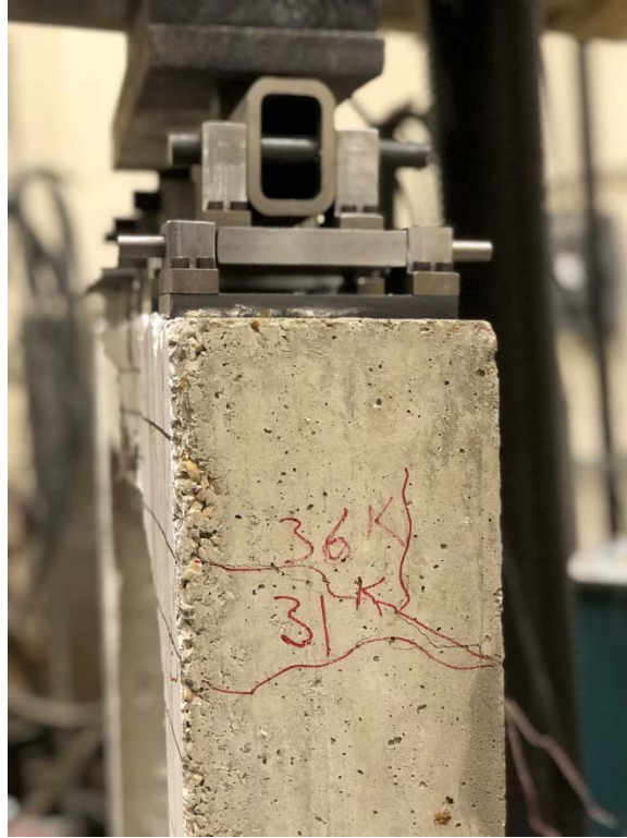
P12. Flexural cracks on the side walls- f'_c = 4.8 ksi
