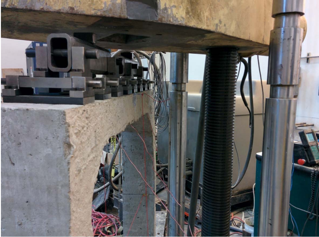
P5. Test setup for first series of test- f'_c = 6.5 ksi
