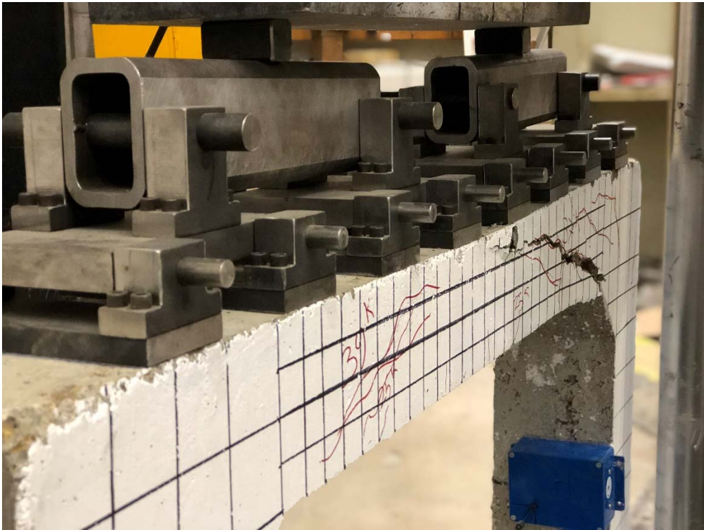
P15. Shear cracking- f'_c = 4.8 ksi (continued)
