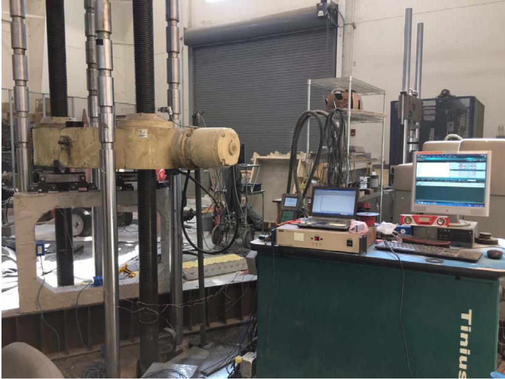
P7. Data Acquisition system- f'_c = 6.5 ksi
