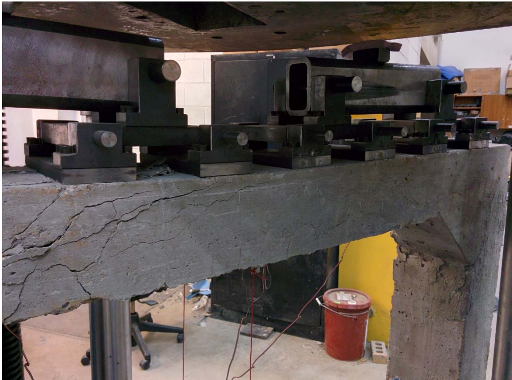
P8. Shear cracking- f'_c = 6.5 ksi
