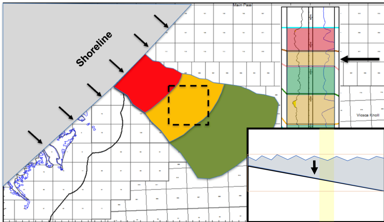
Figure 45. Interpreted environment, movement of shoreline, and water depth for “N-Sand” bed set #4. The colors in the delta figure represent the three different environments with red being the “clean” zone, yellow being the transitional zone, and green being the prodelta. The grey area represents the shoreline, and the arrows represent the interpreted movement that deposited the sediments within the bed set. The box in the right bottom corner represents interpreted sea level, with the highlighted zone being the study area and the arrow representing the interpreted change in water depth resulting in the deposition of the bed set.
