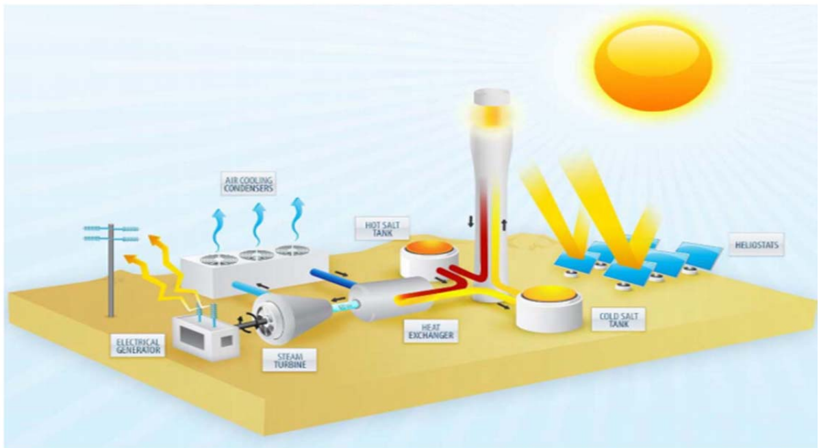
Figure 1.6 Power tower system [12]
