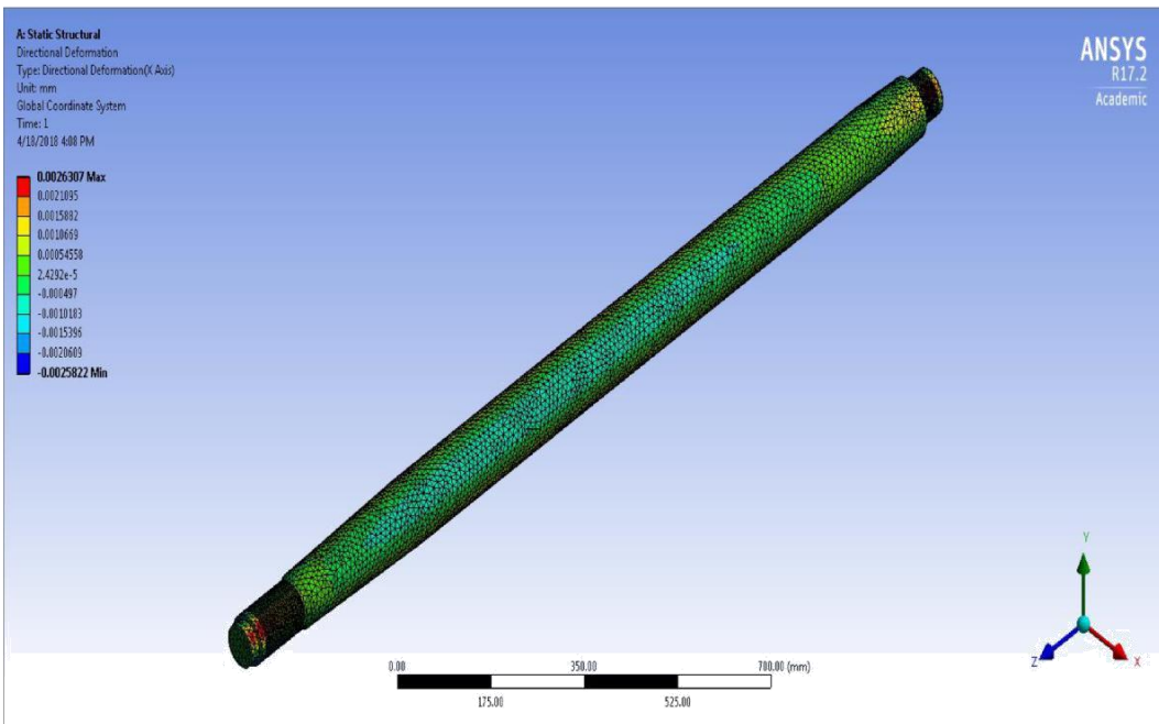
Figure 12 (a) (b) Deformation in metal shaft
