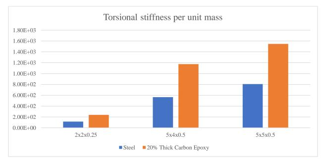
Figure 6-7 Specific Torsional Stiffness
