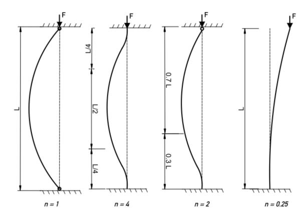
Figure 4-1 Buckling End Conditions
