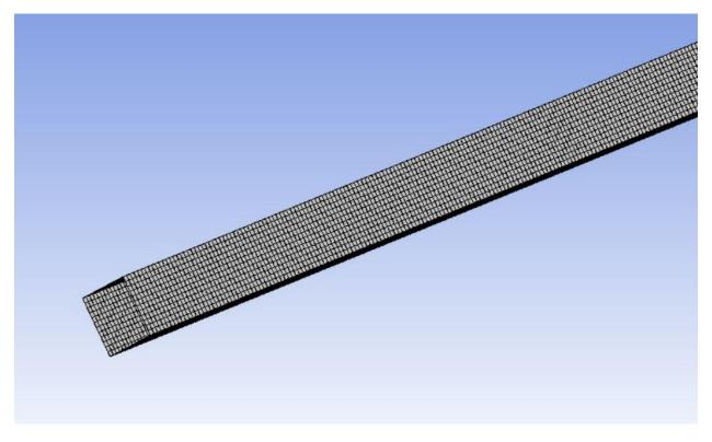
Figure 5-6 Surface Mesh Generated
