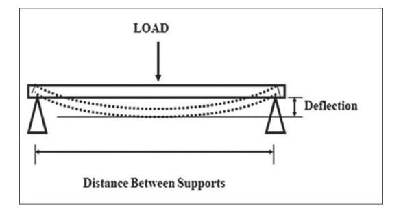
Figure 4-3 Three Point Bend Test
