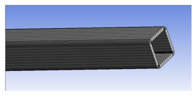
Figure 5-5 Solid Mesh Generated
