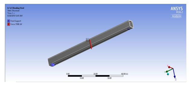
Figure 4-4 Bending Boundary Condition (a)
