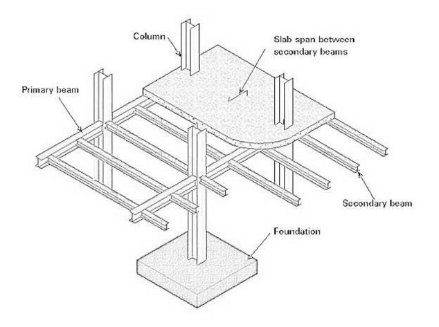
Figure 1-1 Typical Structural Frame
