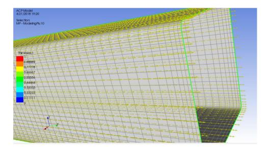
Figure 5-7 Reference Fiber Direction
