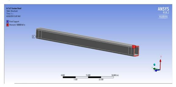
Figure 4-7 Torsion Boundary Condition
