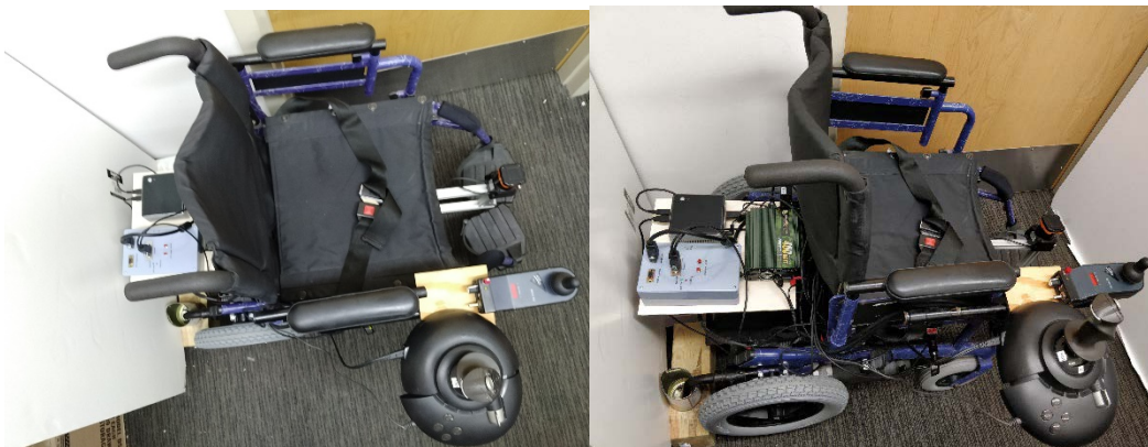
Figure 4-8 Inverter, Intel NUC and the control box mounting
