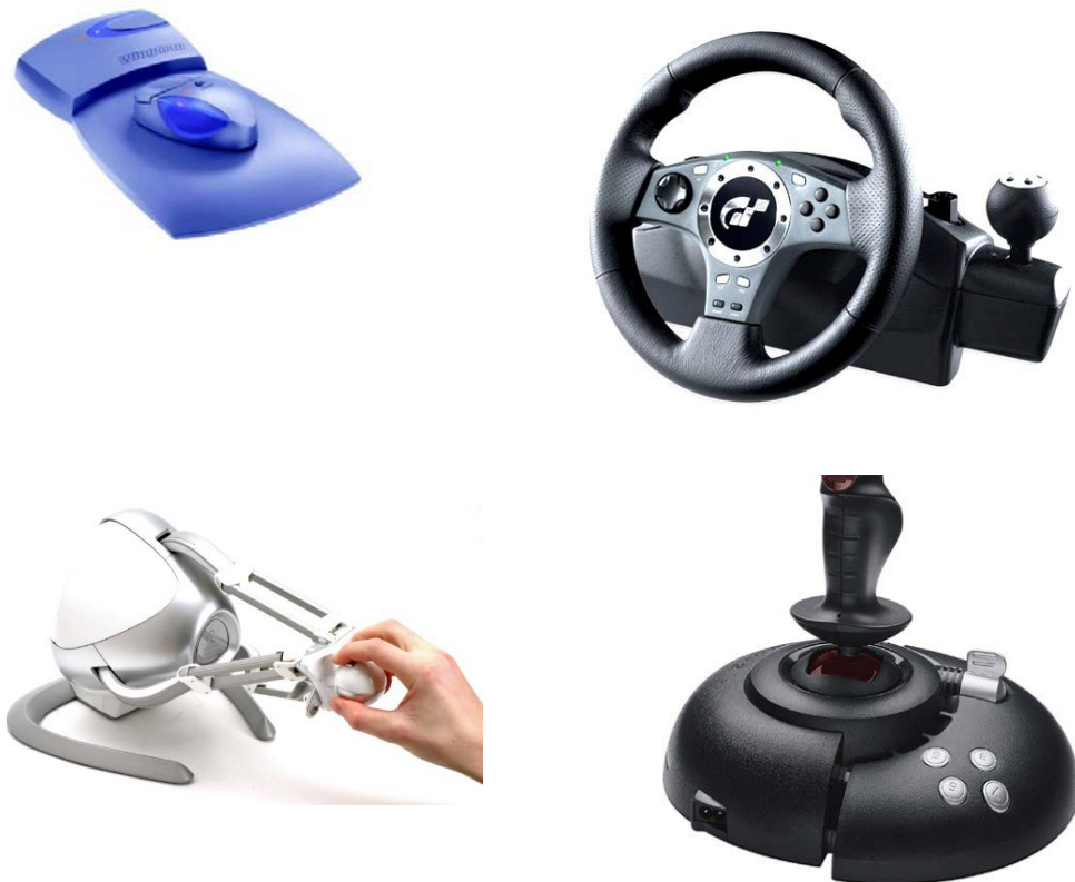
Figure 2-1 Various Force-feedback devices. Top left: Mouse, Right: Steering control; Bottom left: Novint Falcon, Right: Microsoft Force-feedback joystick
