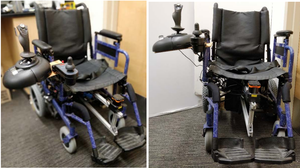
Figure 4-7 Joystick and LIDAR mounting
