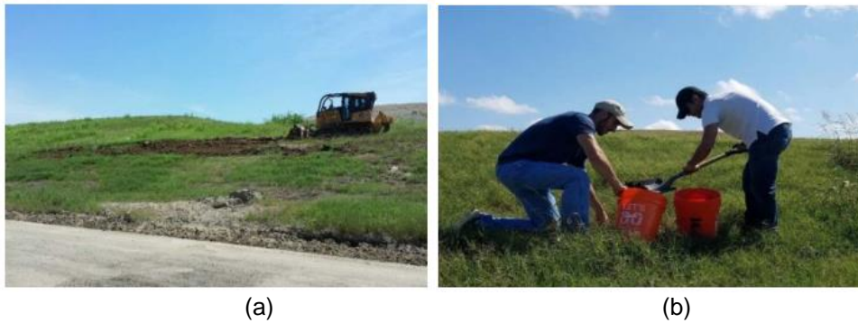
Figure 3.3 (a) Excavation of soil sample from side Slope 1 (b) Collection of soil sample 3.3.1 Geotechnical Properties of soil
