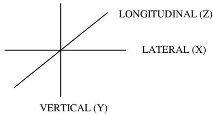
Figure 3.8 Three Axes, Six Degrees of Freedom.
