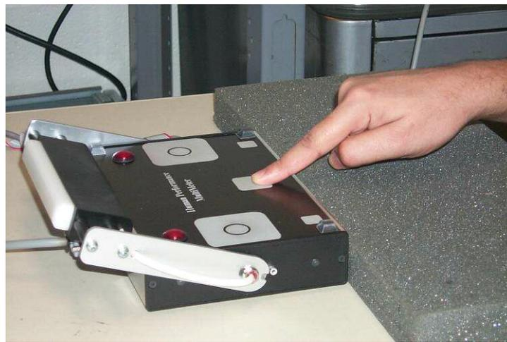
Figure 4.1 Finger Position Before LEDs Turn On in Visual Response Speed Test.
