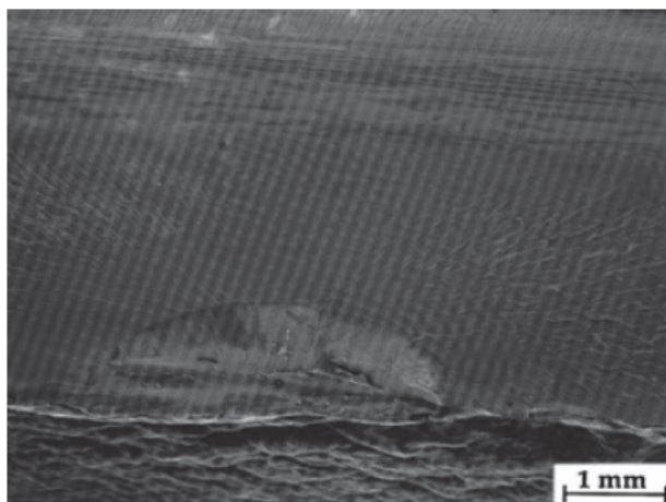
Figure 3-2 Thumbnail Crack Produced in a PE Pipe, Hsuan et al. (2005)
