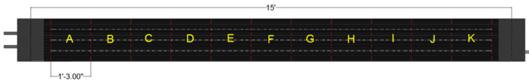
Figure 4-10 Schematic Drawing of Longitudinal Marking of the Pipe Sample
