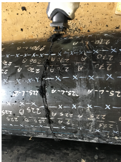
Figure A-1 Reciprocating Saw to Cut the Pipe and Cutting Process
