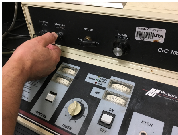
Figure 4-36 Process of Metal-Coating HDPE Specimens (Steps 7 and 8)
