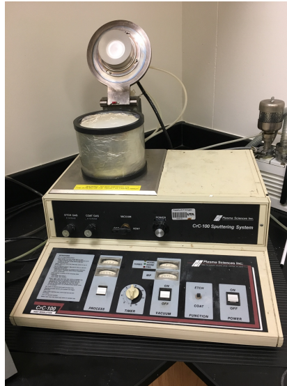
Figure 4-34 CrC-100 Sputtering System
