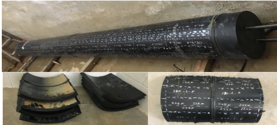
Figure 4-8 Longitudinal and Circumferential Marking of the Pipe Sample
