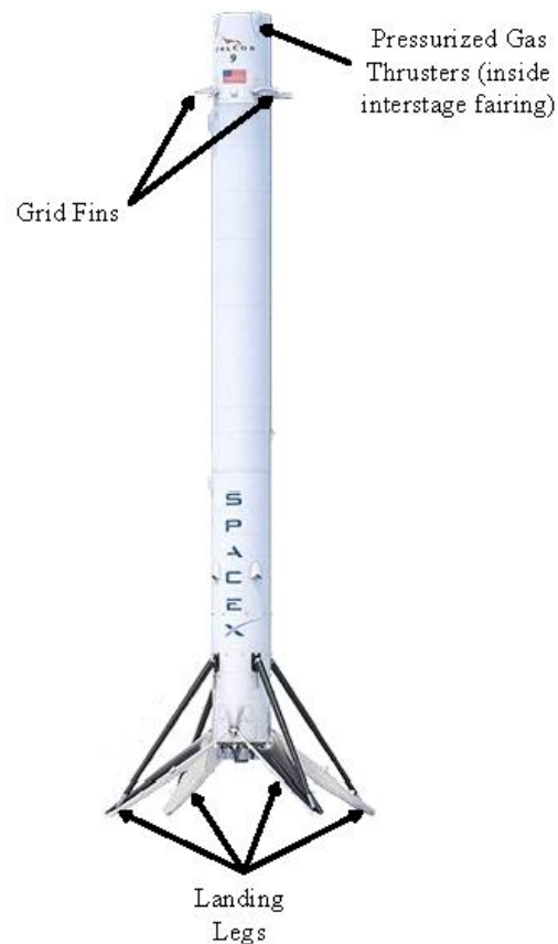
Figure 4.18 Falcon 9 First Stage Landing Hardware [190]
