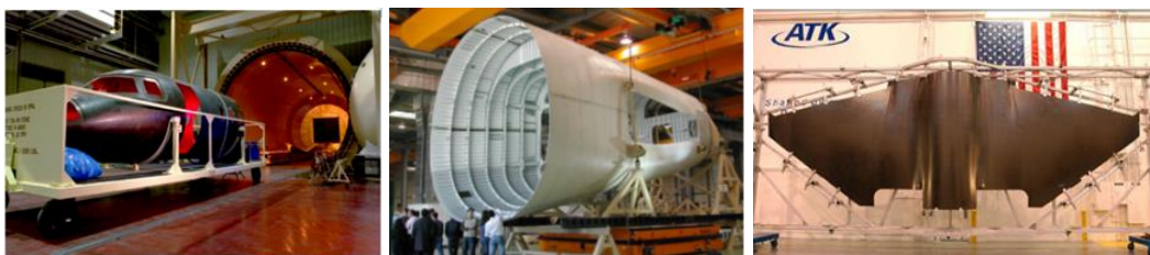
Figure 1-8. Aircraft structures produced using AFP (a) Raytheon business jet fuselage [27], (b) Airbus A380 aft fuselage [28], (c) Lockheed Martin JSF F-35 wing skin [29].
