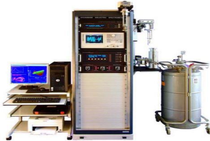
Figure 3-2: Novocontrol Broadband Dielectric/Impedance Spectrometer experimental setup [24]
