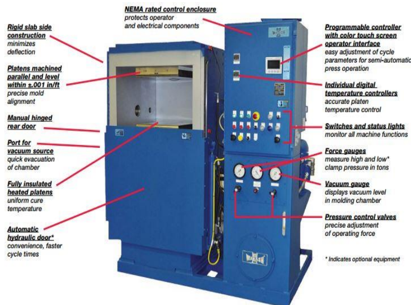
Figure 3-1: Wabash Vantage Series Hydraulic Press for compression molding
