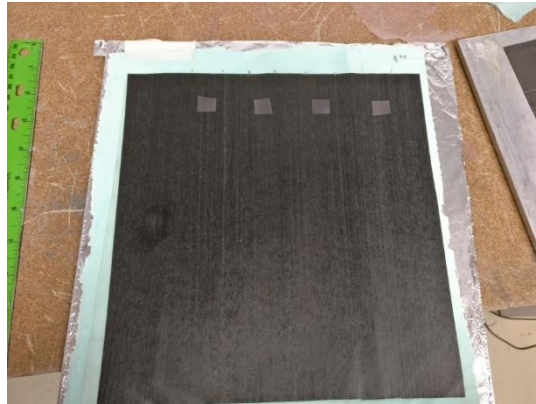
Figure 7-2: Layup of hybrid unidirectional composite with vacuum bagging film as an inclusion/defect
