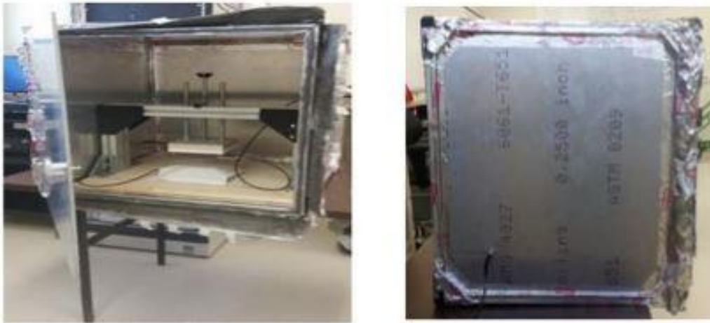
Figure 3-3: Faraday cage setup
