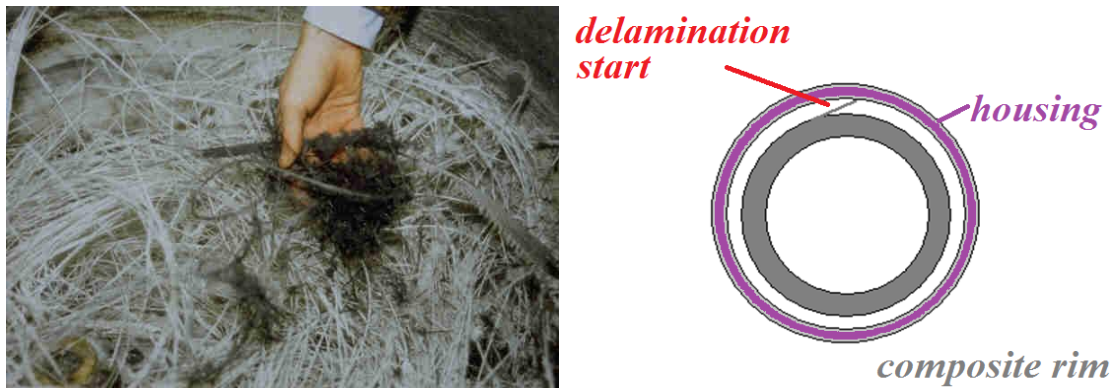
Figure 6-Failure Mode of Composite Flywheel
