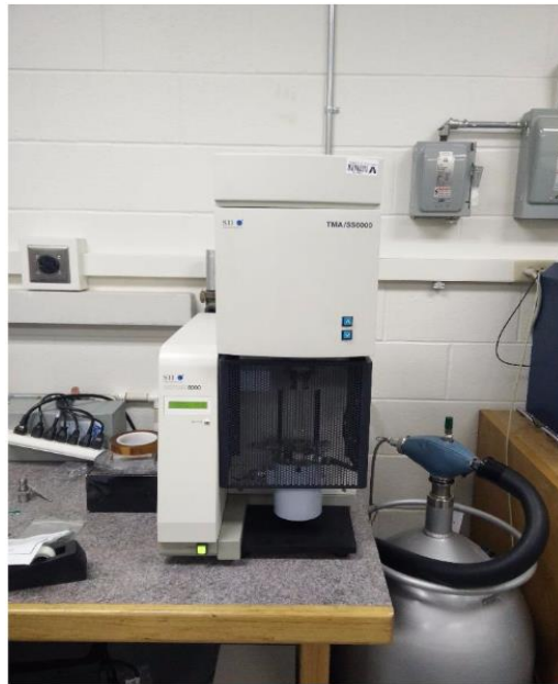
Figure 3.1: Thermo-Mechanical Analyzer (TMA-S6600)
