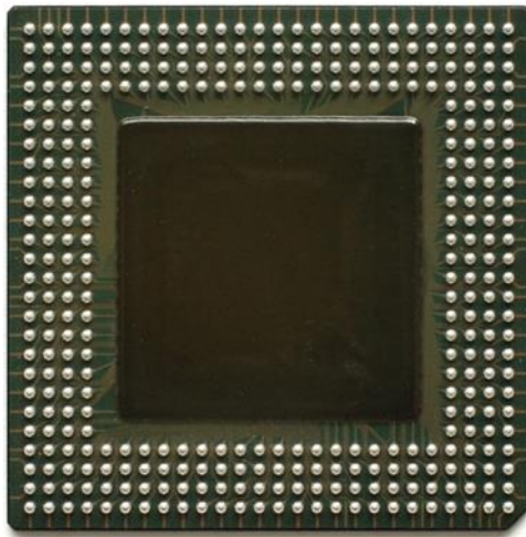
Figure 1.3: Ball Grid Array Package (BGA)
