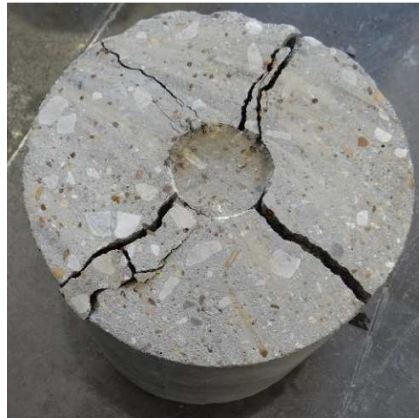
Figure 9-3: Multiple Tensile Cracks Occur Along Diametric Planes of Typical FRC Specimens
