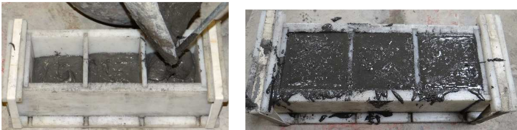
Figure 3-13: Preparation of 2.78 in. cube for UHP-FRC mix
