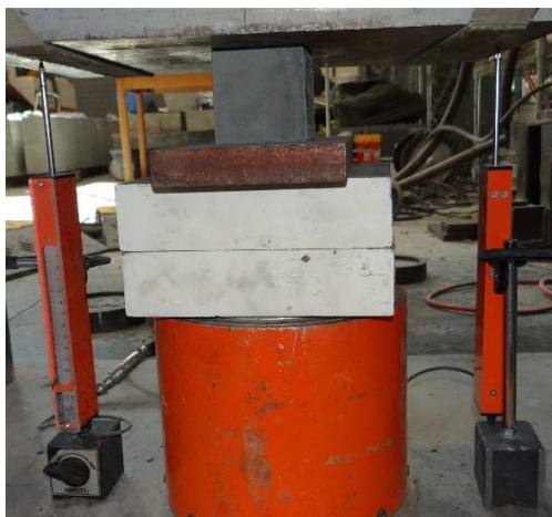
Figure 3-14 Compressive strength test of UHP-FRC (2.78 in. cube)
