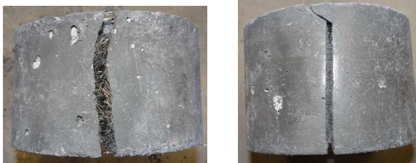
Figure 4-37: Side view (a) 6 x 4 in. (UHP-FRC with steel fibers) (b) 6 x 4 in. (UHP-FRC with PE fibers)
