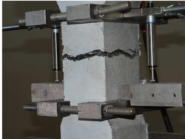
Figure 3-22: Crack location in direct tensile test
