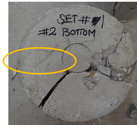
Figure 9-4: Cracks that do not grow up to mid height does not count.
