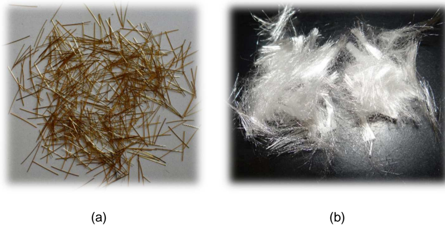
Figure 3-5 (a) Micro-straight steel fibers (b) Polyethylene (PE) fibers
