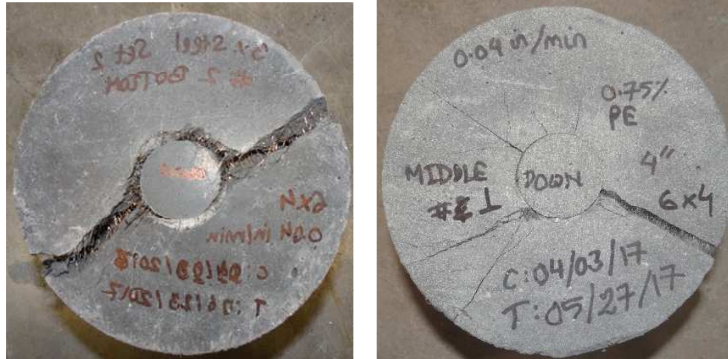
(a) (b) Figure 4-36: Plan view (a) 6 x 4 in. (UHP-FRC with steel fibers) (b) 6 x 4 in. (UHP-FRC with PE fibers)
