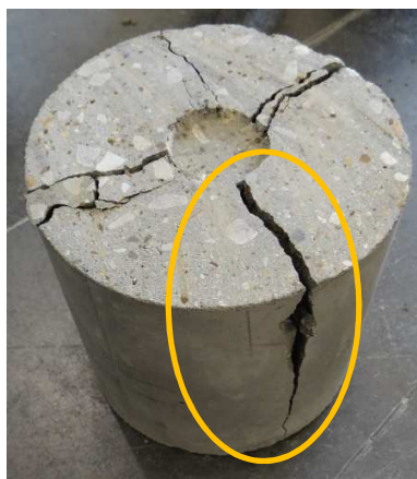
Figure 9-5: Cracks that grow at least up to mid height or full height counts
