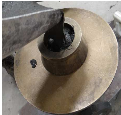
Figure 3-16 Flow table apparatus in accordance to ASTM C230 (2014)
