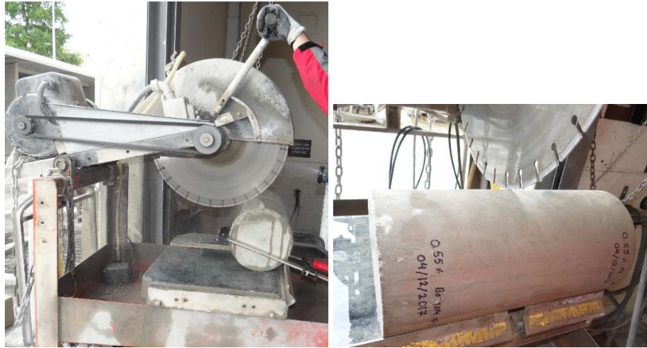
Figure 3-12 Preparation of DPT specimen using a concrete saw
