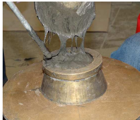
Figure 3-16 Flow table apparatus in accordance to ASTM C230 (2014)
