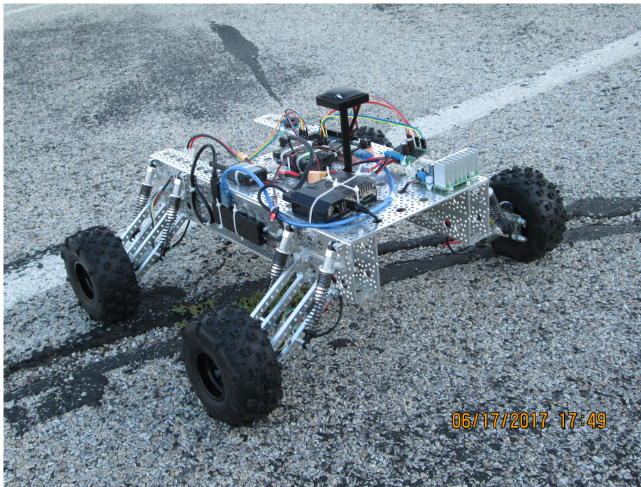
Figure 5.1: Differential-drive robot built at Aerospace Systems Laboratory, UTA
