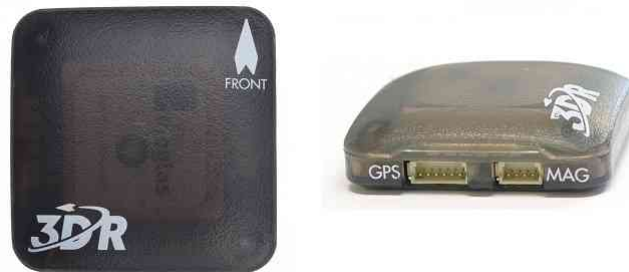
Figure 5.3: 3DR u-blox GPS/Compass used on the ASL-Gremlin-Rover Source: http://ardupilot.org/copter/docs/common-installing-3dr-ublox-gps-compass-module.html
