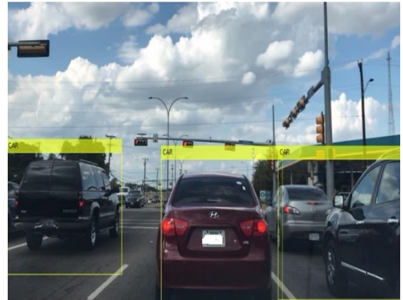
Fig.5.8 Detection Results Faster R-CNN (Result images source– Self generated data set)
