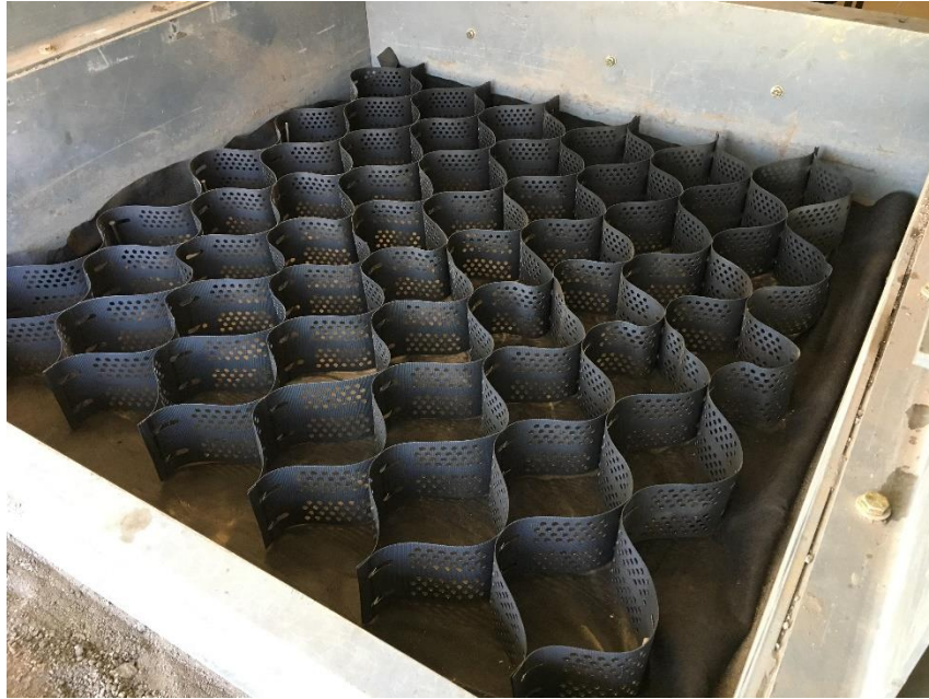
Figure 3.9 Geocell placed in a large testing box
