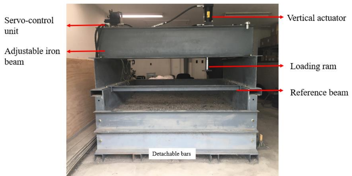
Figure 3.11 Front of the large testing box
