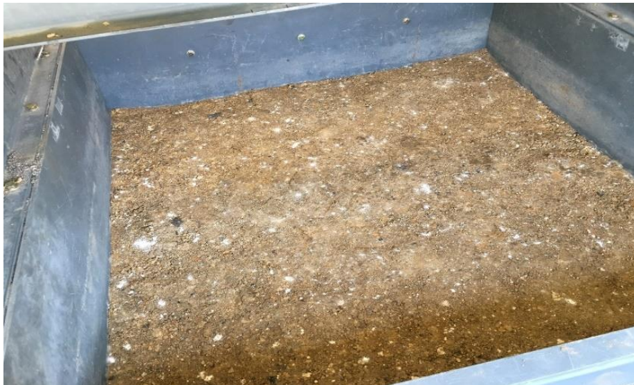
Figure 3.22 Compacted subgrade in the large testing box
