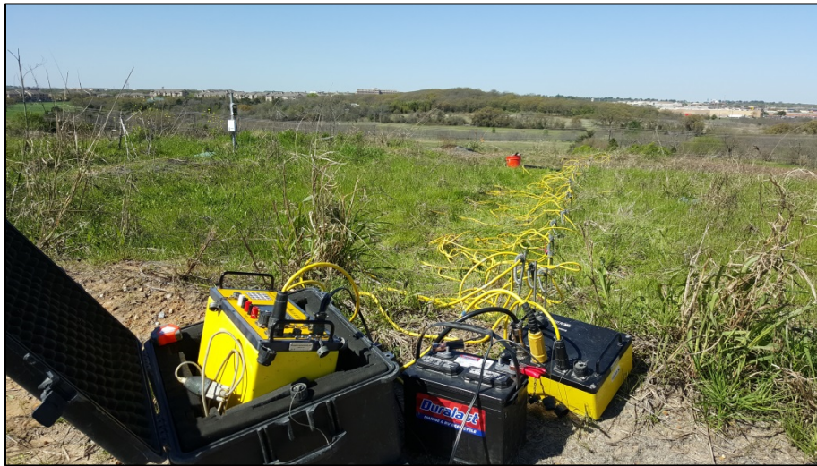
Figure 5-3 Electrical resistivity imaging along the lysimeters
