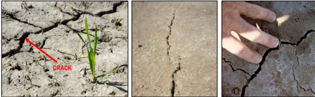
Figure 2.2 Failure mode of prescriptive landfill cover
