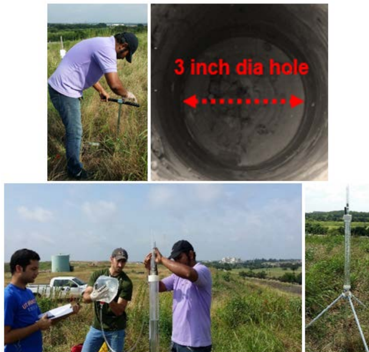
Figure 3.31 In-situ hydraulic conductivity test using GP
