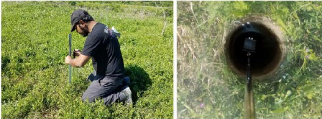
Figure 3.20 Root observation using telescopic inspection mirror
