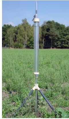
Figure 2.39 In-situ hydraulic conductivity measurement with GP
