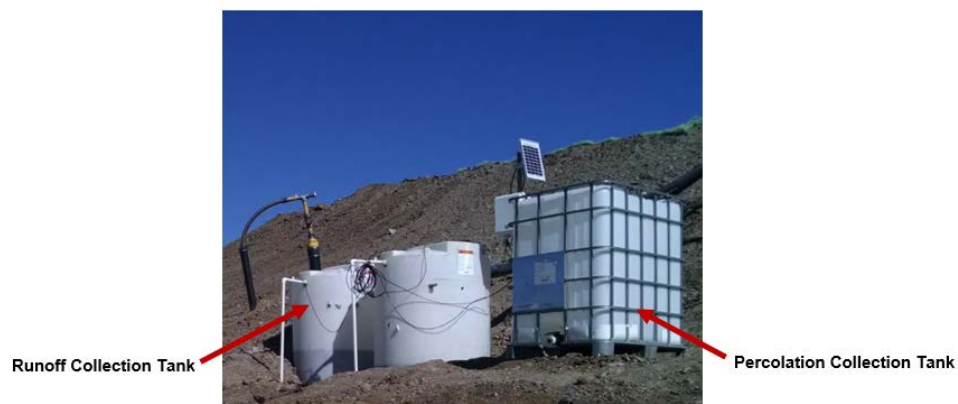
Figure 3.4 Surface runoff and percolation collection tanks in the study area (Modified from Brett Devries, 2016)
