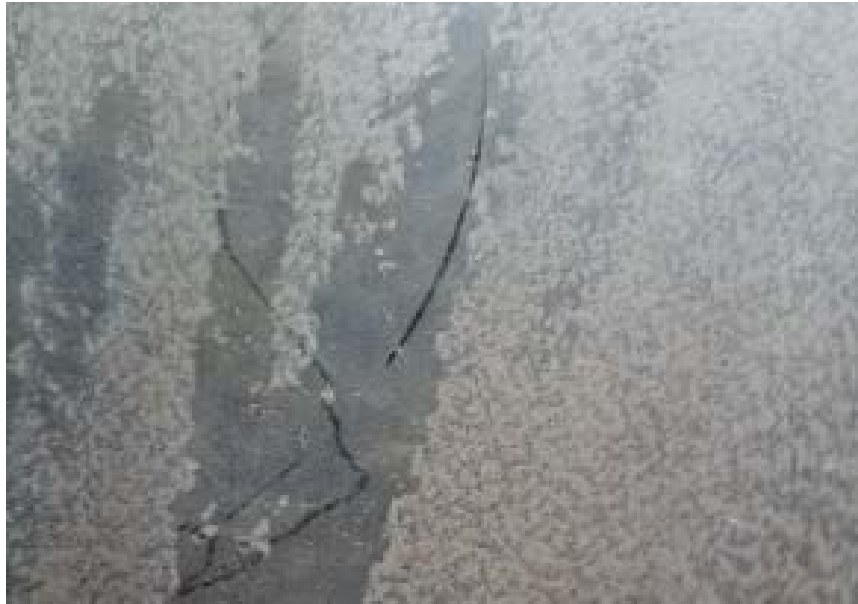
Figure 5.31 Blurred image (soil accumulation at the interface of the outside minirhizotron wall and soil cover)
