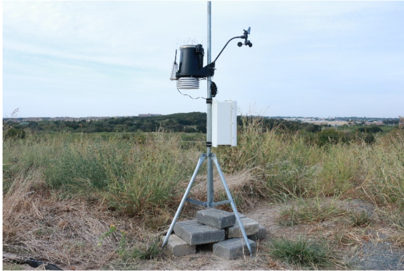
Figure 3.5 On-site weather station
