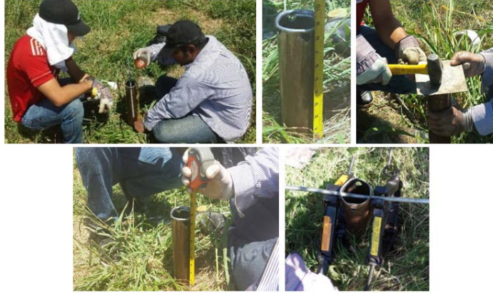
Figure 3.29 Destructive sample collection for RMD test
