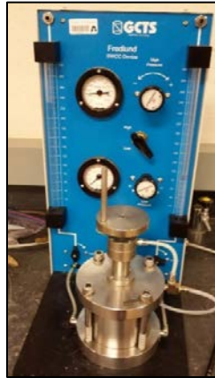
Figure 3.9 Pressure cell apparatus (Fredlund SWCC Device)
