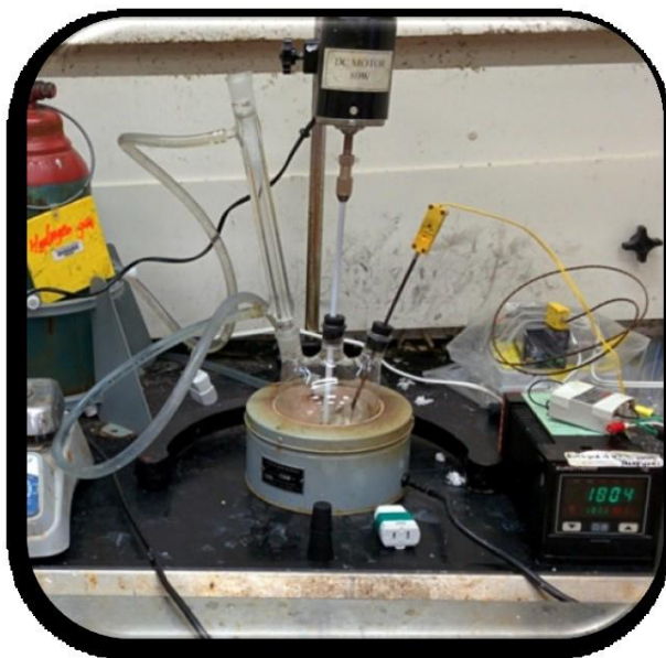
Figure 3-3: Experimental setup for synthesis of the polymer
