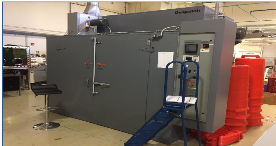
Figure 3: Oven with vacuum lines and thermocouple, IPPM, UTARI
