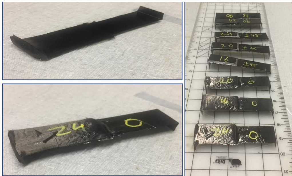
Figure 32(a): Coupons with restricted edges after cure
