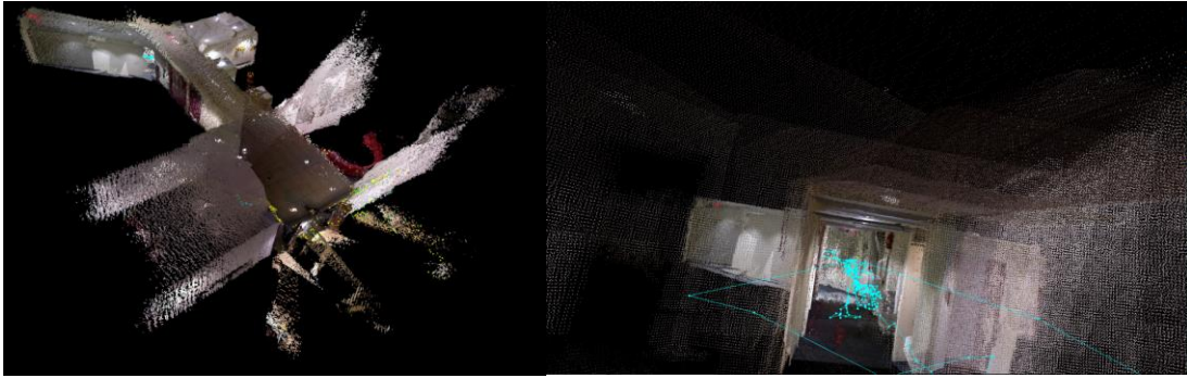
Fig 11. Dimensional Pointcloud maps using real time appearance based mapping (Left: UTARI Atrium, Right: Navigation within the 3D map and odometry in blue)
