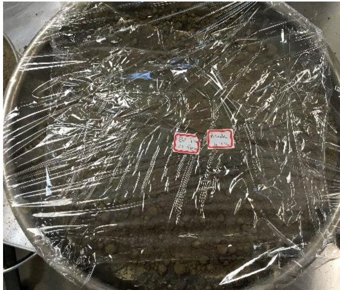
Figure Error! No text of specified style in document.-20: Soil mixture wrapped with plastic bag for mellowing
