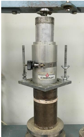
Figure Error! No text of specified style in document. -21: Triaxial loading frame
