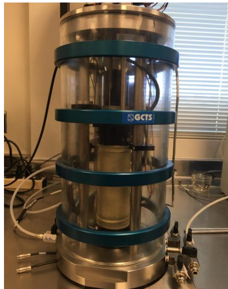
Figure Error! No text of specified style in document.-9: Acrylic plastic reinforcement for the cell
