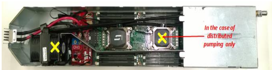
Figure 4-22: Server 123 showing location of fan and pump that are not powered in distributed pumping case
