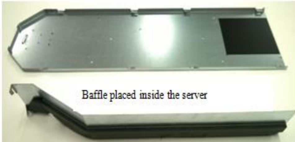
Figure 4-2: Cover with ducting for the server
