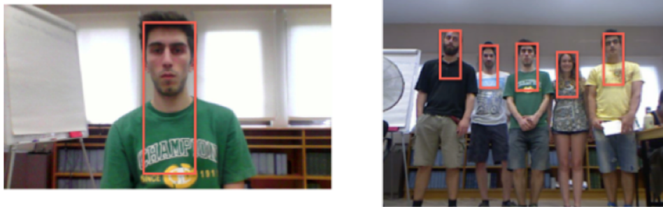
Figure 7.7: Face detection examples captured from the application and from Kinect camera of the robot.
