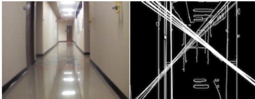
Figure 7.14: Image after the Canny edge detector and have been applied the Hough transform algorithms.
