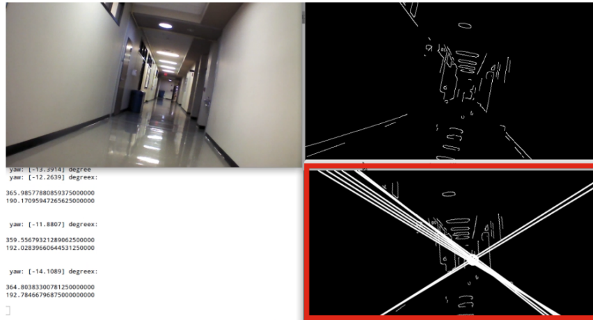
Figure 7.19: Compensate the yaw angles of the AR.Drone with the captured images.
