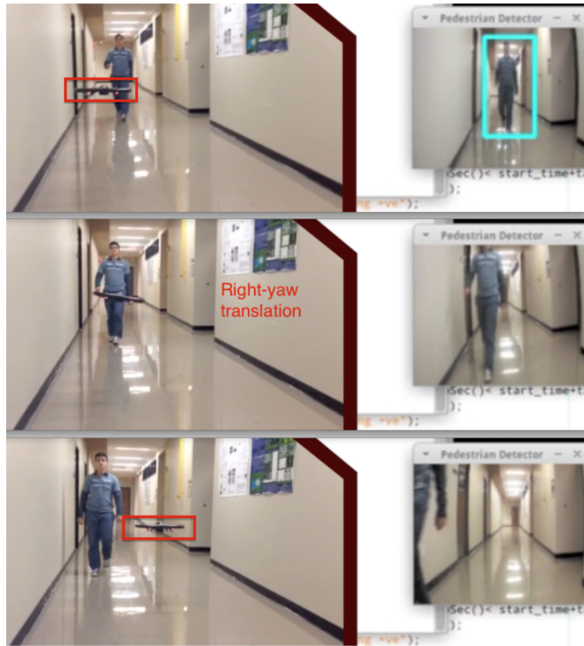
Figure 7.18: Sequence of frames that show the AR.Drone position (red rectangle) when detects a human being in front of it and try to avoid him.
