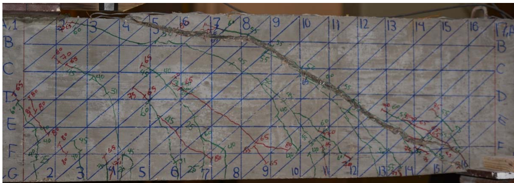
Figure 4.176 A view of failure in beam SFRC18b
