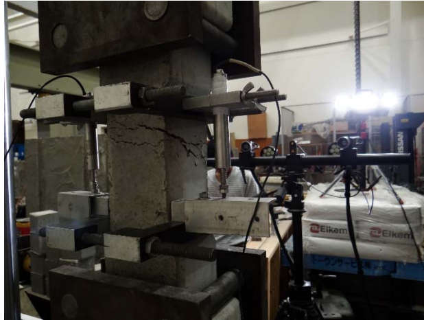
Figure 3.35 DIC system measuring the width of crack for dog-bone shape specimen
