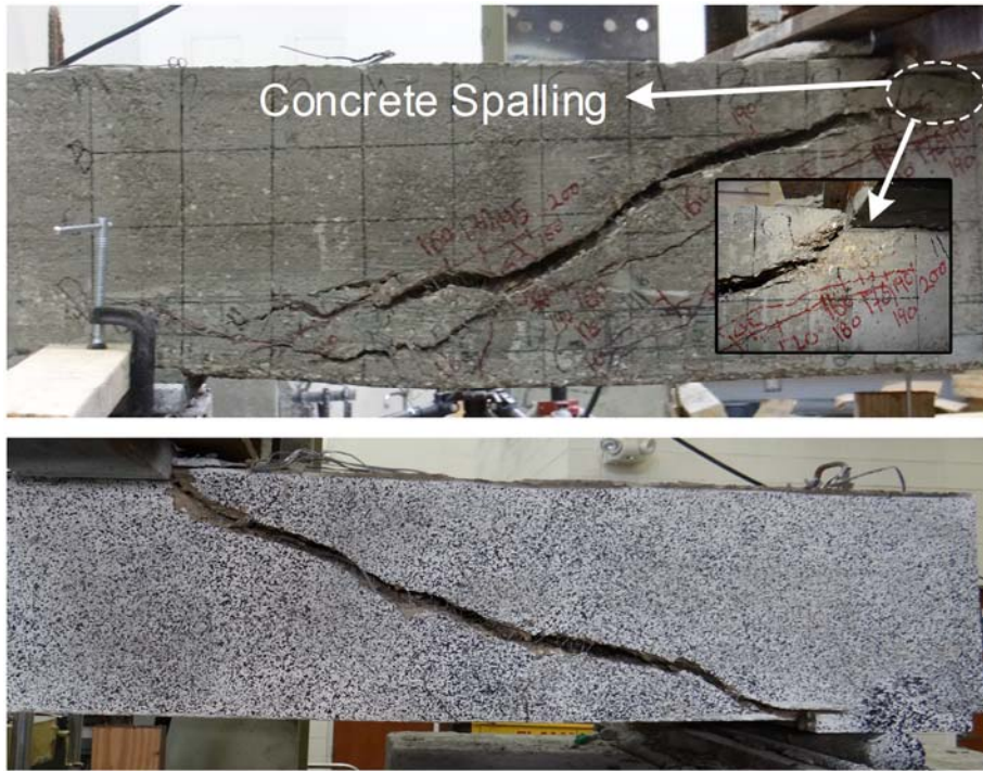
Figure 4.107 A view of failure on both sides of beam SFRC 12W24
