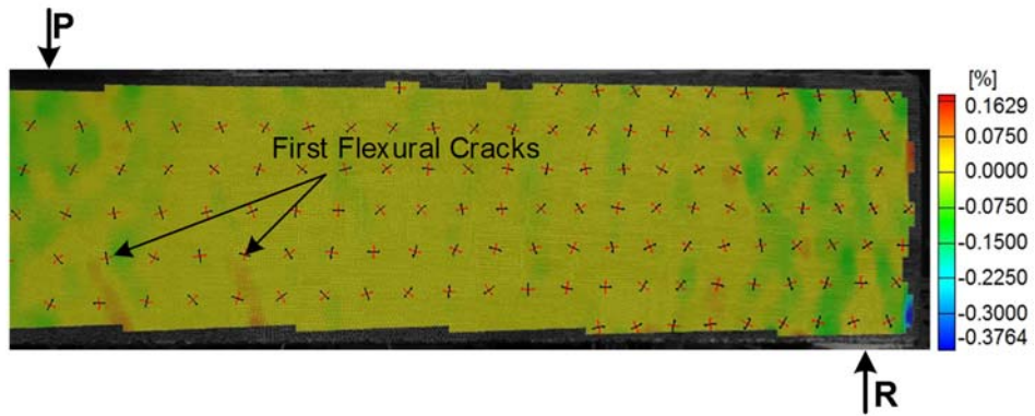
Figure 4.34 Full-field concrete longitudinal strain ( \epsilon_x ) across shear span for specimen RC18b at load 10 kips
