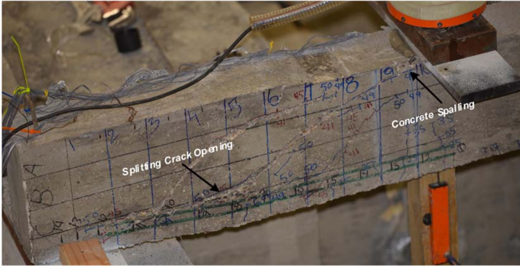
Figure 4.67 Formation of splitting crack at the level of flexural bars as a post-peak phenomenon
