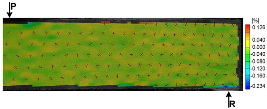
Figure 4.35 Full-field concrete transvers strain ( \epsilon_y ) across shear span for specimen RC18b at load 10 kips
