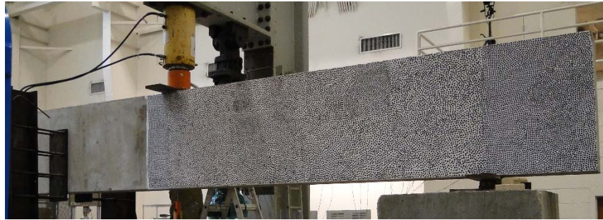
Figure 3.22 Spackle pattern created by stamping black paint dot on white base (specimen SFRC36b)
