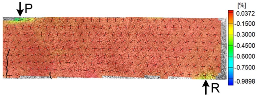
Figure 4.131 Full-field concrete minimum principal strain ( \sigma_2 ) across shear span for specimen SFRC12W24 at normalized shear stress of 2.5\sqrt{f'_c} .
