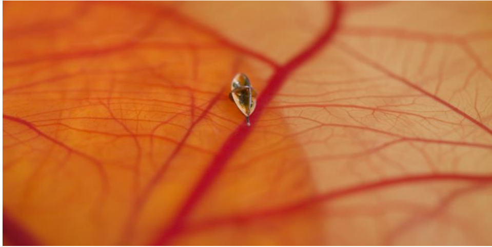
Figure 2-1. 2 mm long microrobot with a needle to puncture vasculature on a CAM [71].
