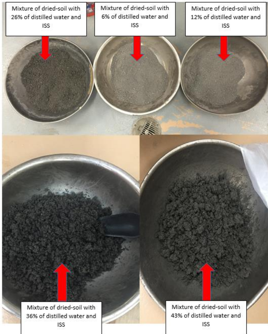
Figure 3. 10 Prepared stabilized soil
