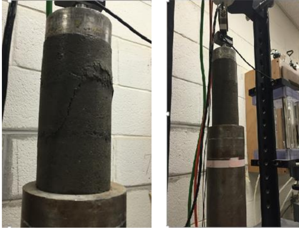
Figure 3. 14 Soil sample a) before failure b) failure plane
