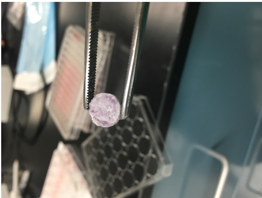
Fig 4.19 precipitated of formazan on the scaffold
