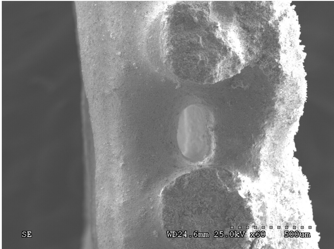
Fig 5.6 The cross-section area of porous scaffold
