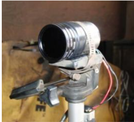
Figure 2-15 Light Measurement Device with ND Filter
