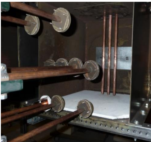
Figure 2-6 Vertical Electrodes in the Cubic Box (VCBB), Electrodes are Terminated at the Bottom of the Box
