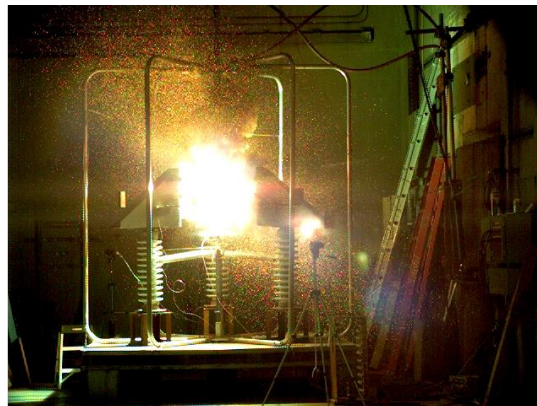
Figure 1-5 Ejection of Metal Particles in an Arc Flash Test
