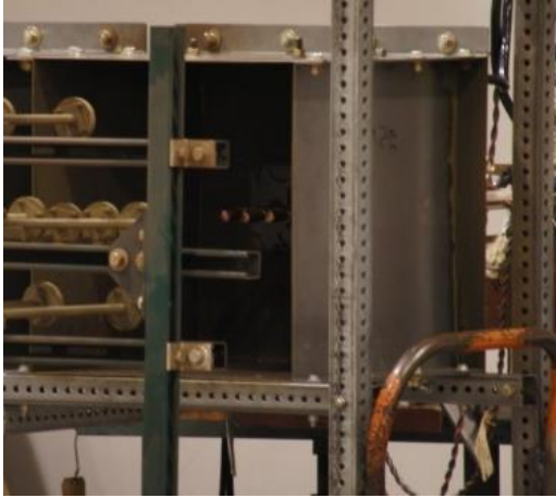
Figure 2-7 Horizontal Electrodes in the Cubic Box (HCB)
