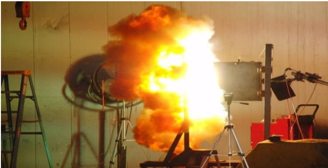
Figure 1-1 Three Phase Arc Flash Event in the Enclosure
