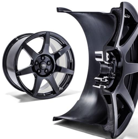
Figure 2-10 Cross section of Shelby GT350R's carbon wheels.
