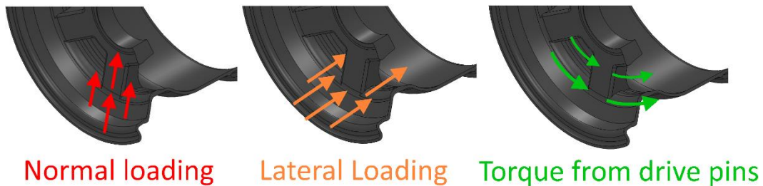
Figure 3-10 Load paths along the wheel spokes
