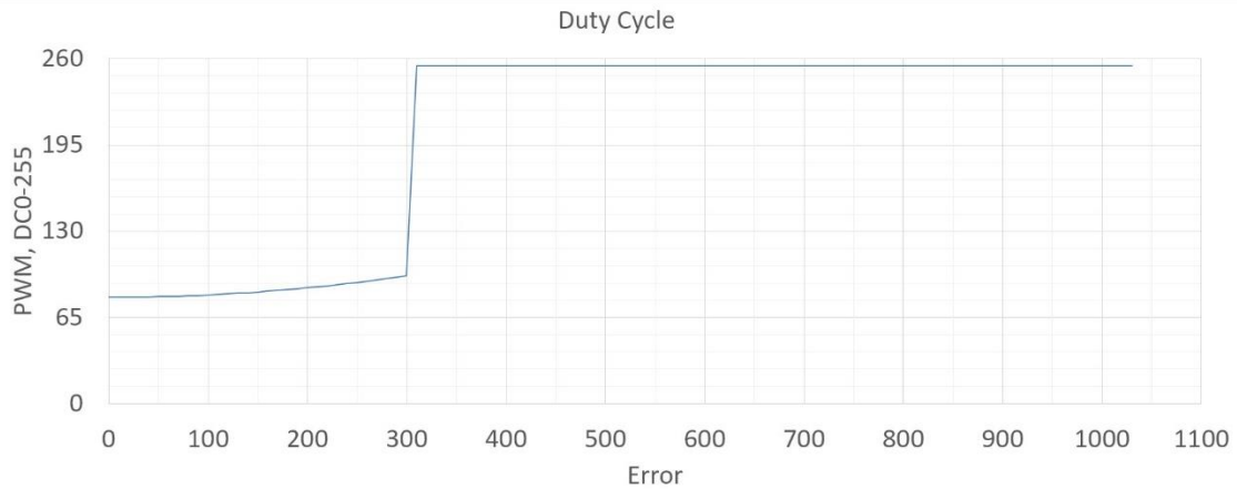
Figure 11 PWM duty cycle logic for clutch for positive error
