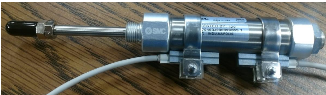
Figure 18 Shift cylinder with reed switch installed
