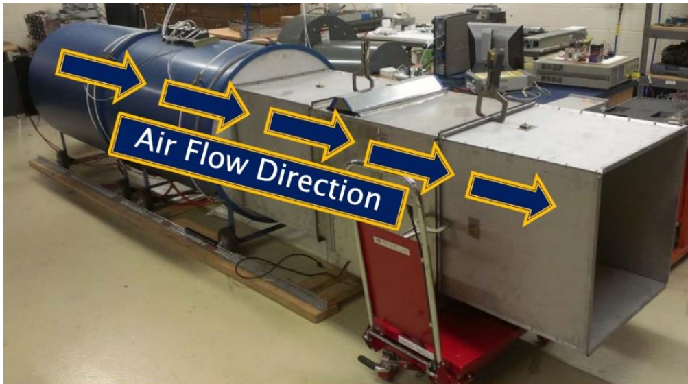
Figure 2-1 Air Flow Bench Set-up [2]
