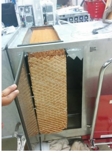
Figure 2-3 Wet Cooling Media
