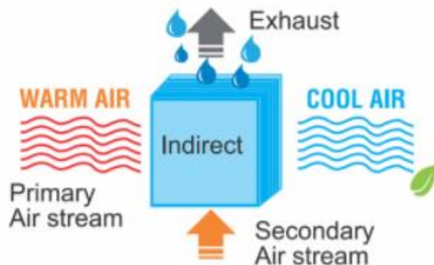
Figure 1-4 In-direct Evaporative Cooling [5]
