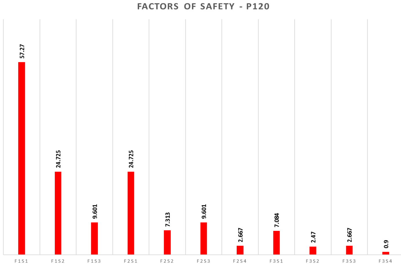
Figure 4-3 (c) Calculated factors of safety for P120 Carbon/epoxy
