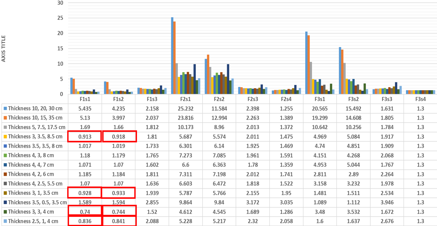
FOS OF COMPOUND LAYERS WITH DIFFERENT THICKNESSES
