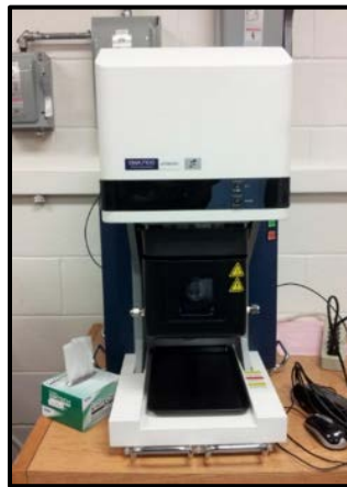
Figure 3.7: Dynamic Mechanical Analyzer (DMA)
