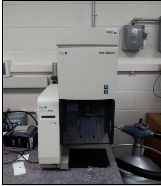
Figure 3.3: Thermo Mechanical Analyzer (TMA)
