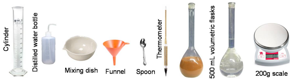
Figure 4-12 Tools used for testing specific gravity of soil
