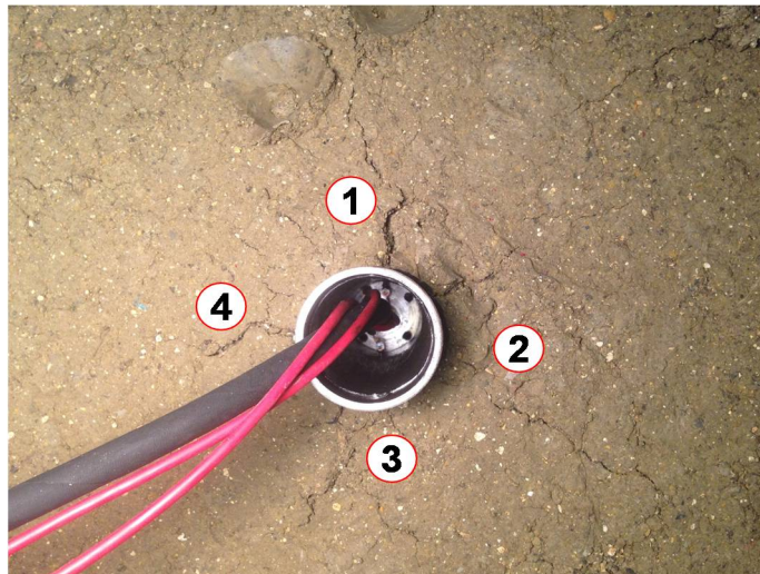
Figure 5-5 Effects of boundary conditions of cone penetration test in first soil chamber
