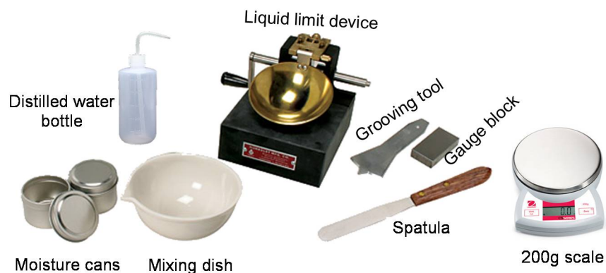
Figure 4-8 Casagrande tools for liquid limit test.
