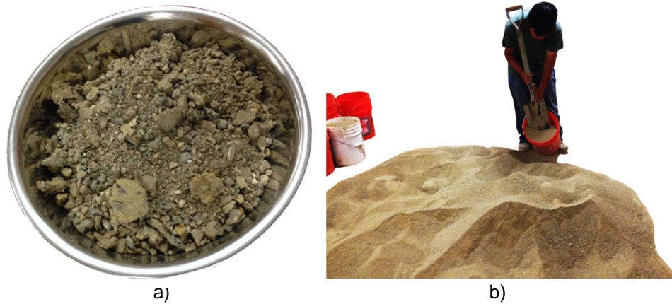
Figure 4-3 Soil preparation: a) Dried soil, b) Soil mixing after crushing
