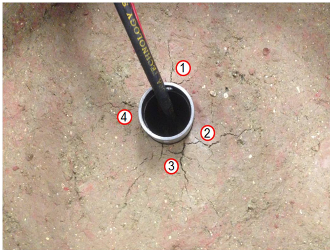
Figure 5-9 Effects of boundary conditions of cone penetration test in third soil chamber
