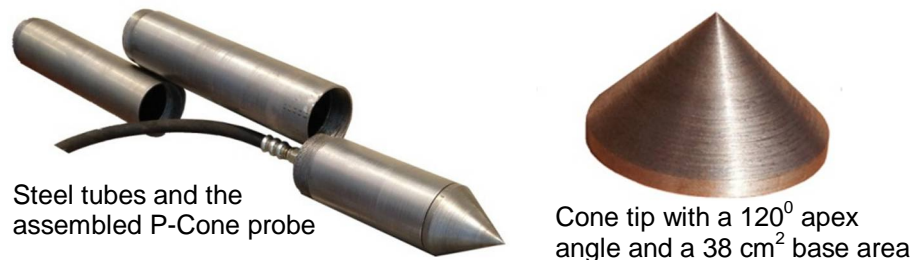
Figure 3-6 Assembled P-Cone probe and the 120^{\circ} cone tip
