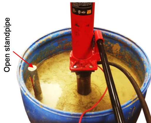
Figure 4-27 Cone penetration test performed 30 days after soil chamber was refilled with water
